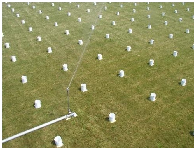
Figure 2. Grid of catch cans.
