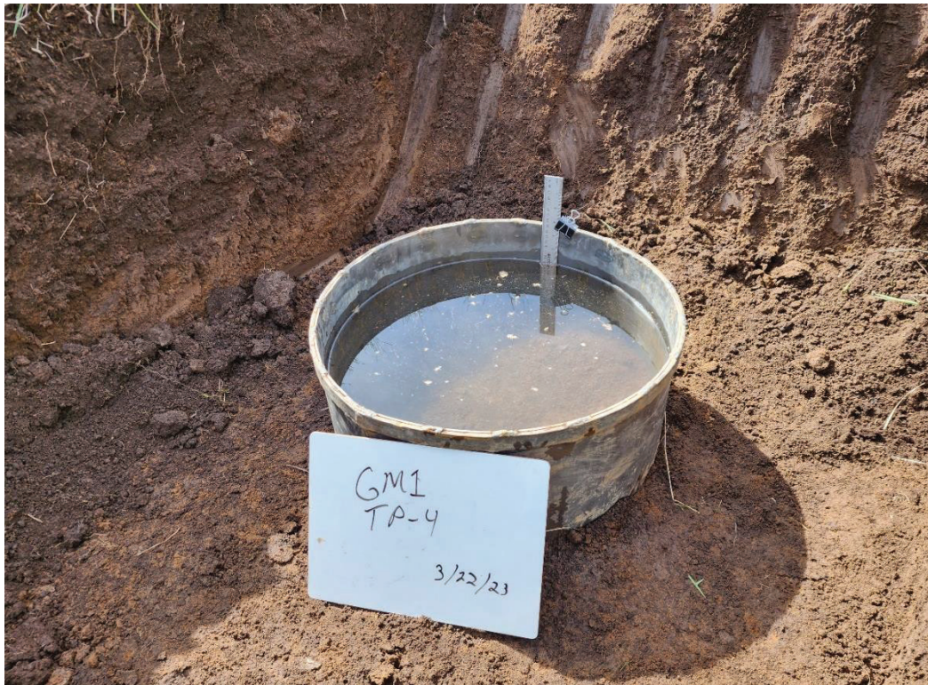
Figure 2. Example CI measurement (GM1, TP-4 at 2 ft bgs)
