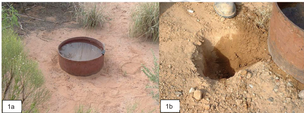
Figure 1. Cylinder infiltrometer testing (1a); measurement of lateral divergence (1b)
