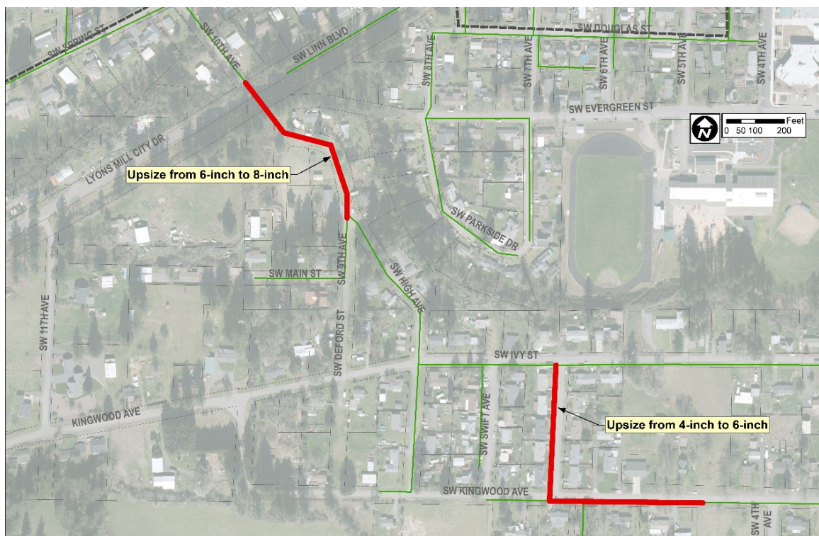
FIGURE 6-4: SPRING STREET BASIN TRUNKLINE UPSIZE
