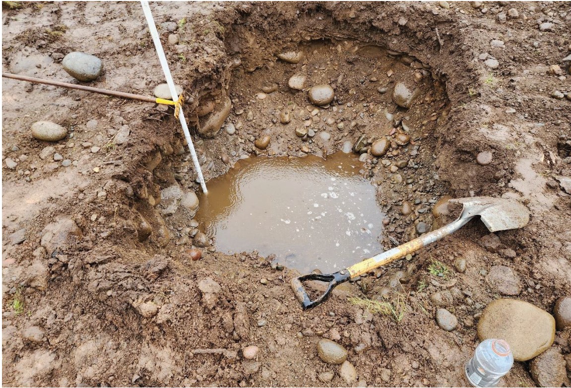
Figure 3. Example modified test pit infiltration measurement (GM1, TP-4 at 3 ft bgs)
