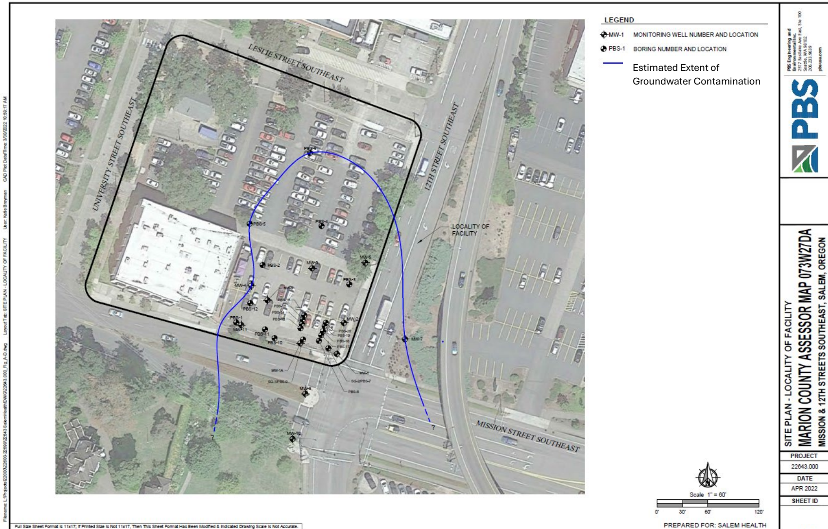
Figure 8: Estimated Extent of Petroleum Contamination in Groundwater
