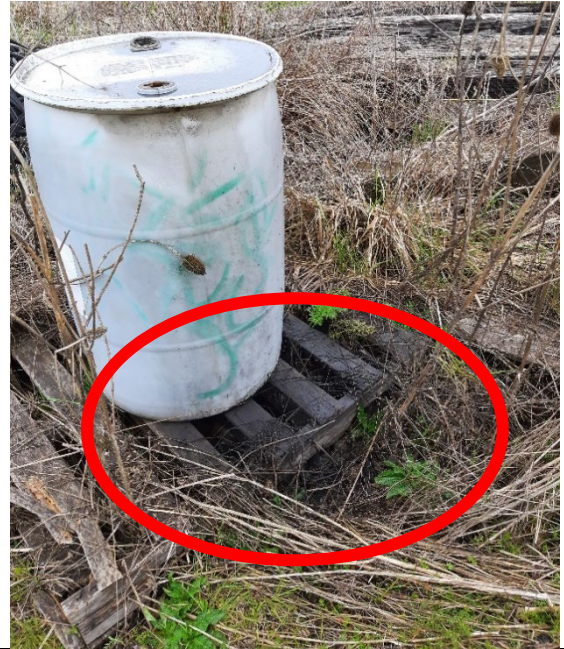
Photo 6: Outside used oil storage area near the AST: Close-up of a container without secondary containment, a label, and used oil leaking onto the ground area highlighted in red.
