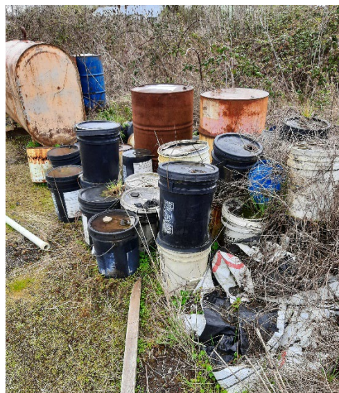
Photo 4: Outside used oil storage area near the AST: Close-up of containers without secondary containment, labels, and multiple containers in poor condition without lids. The containers were observed to contain contents.
