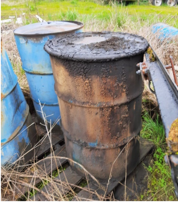
Photo 13: Outside used oil storage area near the AST: Containers in poor condition, without secondary containment, and labels. The containers were observed to contain contents. Photo taken: April 21, 2023
