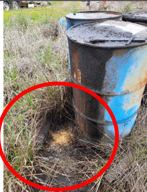
Photo 8: Outside used oil storage area near the AST: Close-up of a container without secondary containment, a label, and used oil leaking onto the ground in the area highlighted in red.
