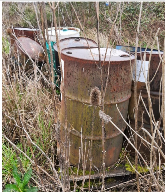
Photo 11: Outside used oil storage area near the AST: Containers without secondary containment, labels, and multiple containers in poor condition. The containers were observed to contain contents.
