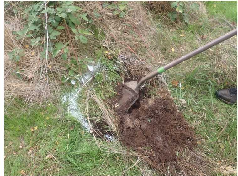
Magnetic anomalies were further investigated, when possible, by exposing the buried feature(s) with a shovel.
