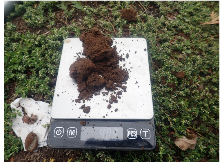
Soil subsamples were weighed in 40g increments before being placed into a glass sample container.
