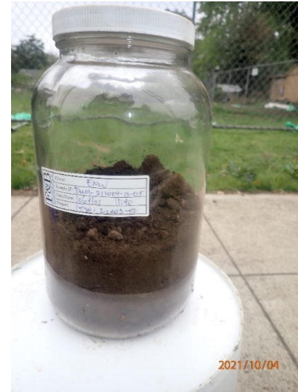
All sample increments from DU01 were placed in a sample jar and uniquely labeled prior to submitting it to the laboratory.
