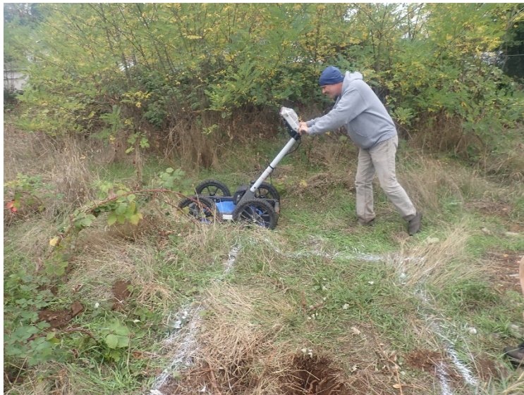
A Ground-Penetrating Radar device was used to scan non-metallic reflections. White paint marks were drawn around buried features of concern
