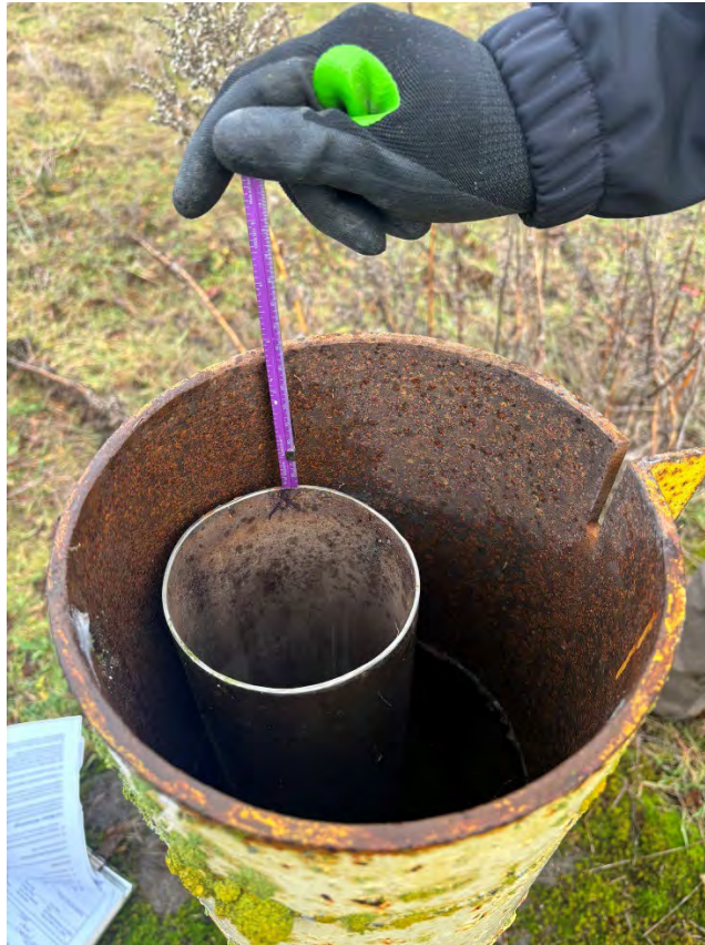
Photograph 7: Measured distance between the inner and outer casing of MW-23d was 2.75 inches, which is similar to recent observations. View facing east.
