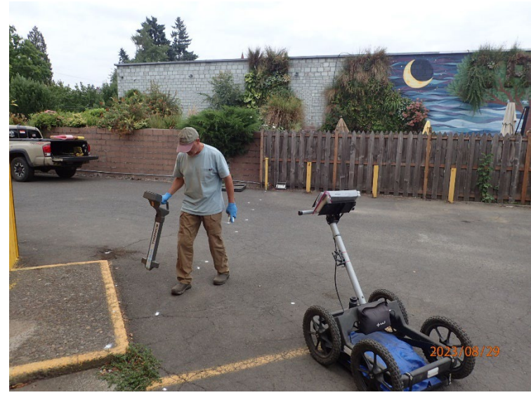
A geophysical survey was conducted to assist in siting location for additional soil boring EB11 south (presumed down gradient) of EB09.
