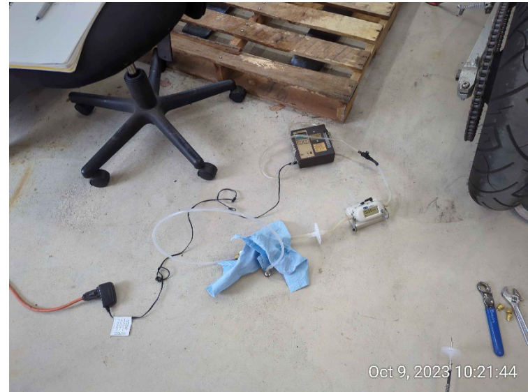
Rags treated with isopropyl alcohol were placed at connections along sample string for leak detection purposes.
