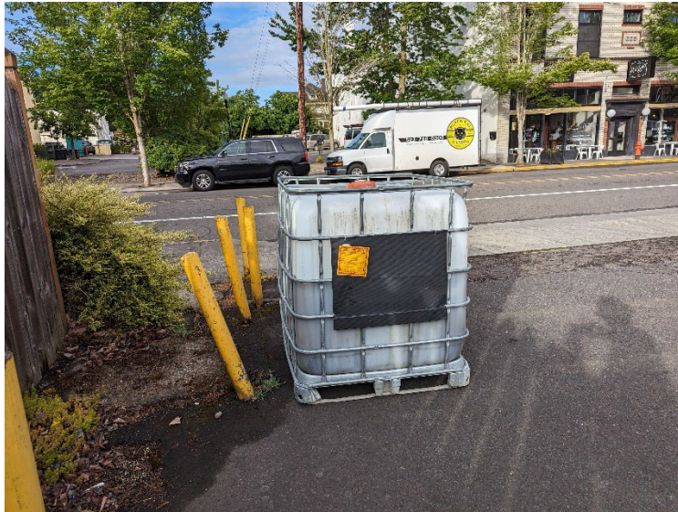
Labeled tote used to store liquid contents of UST01.
