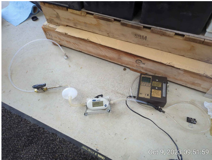
Flow meter and pump set up for TO-17 sampling.
