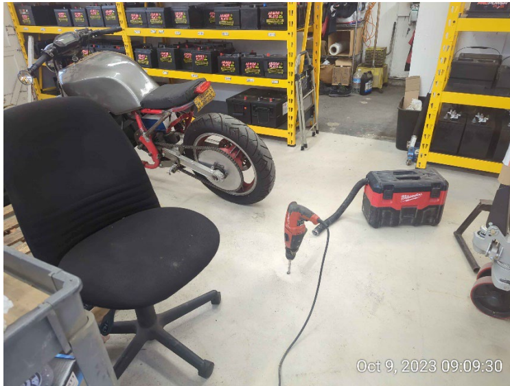
A 5/8-inch hole drilled through building slab floor in preparation of sub-slab vapor sampling.
