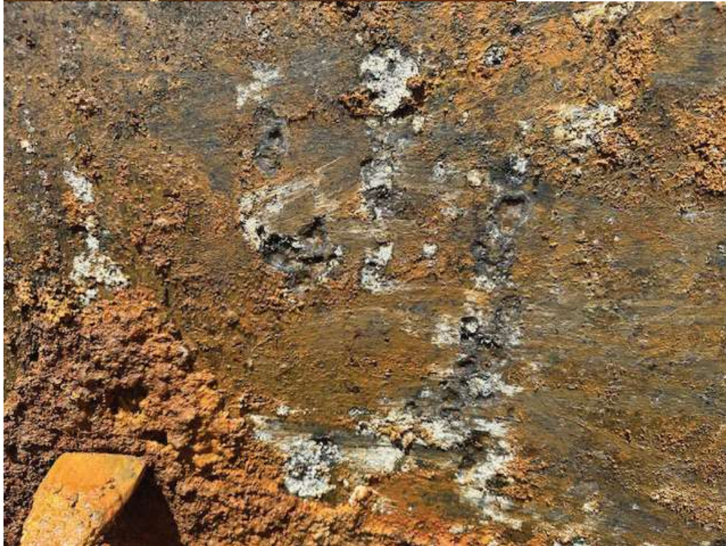
View of the floor of the gas tank. A thick and hard layer of corrosion was strongly attached to the floor of the tank. There were strong corrosion pits, but none of the pits went through the gas tank.
