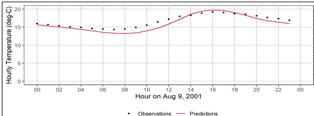
Figure 3-29: Little Sandy River above PGE diversion (river km 3.1): Modeled vs. observed hourly
