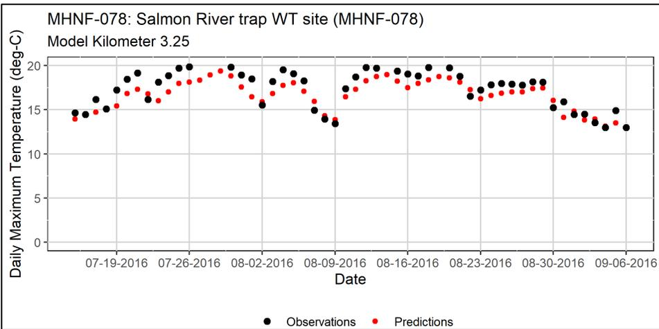
**Figure 3-17: Salmon River trap WT site: Modeled vs. observed daily maximum temperatures.**
