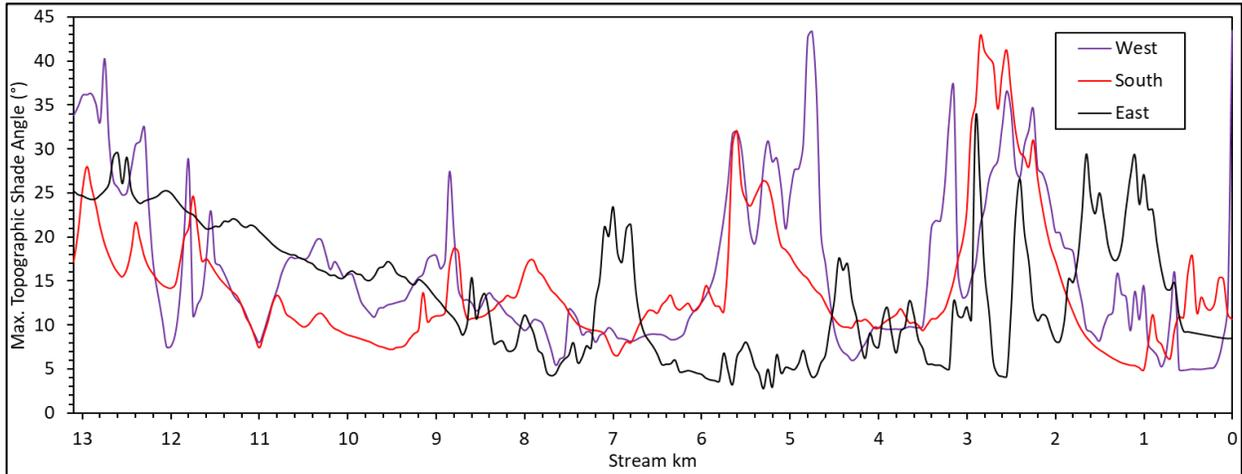
Figure 3-11: Salmon River model inputs: Topographic shade angles.
