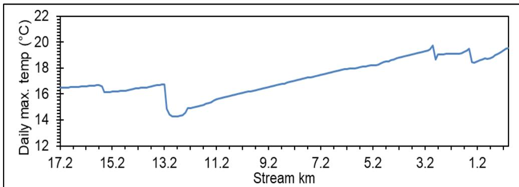
Figure 3-33: Little Sandy River model results: Longitudinal daily maximum temperatures, 8/9/2001.
