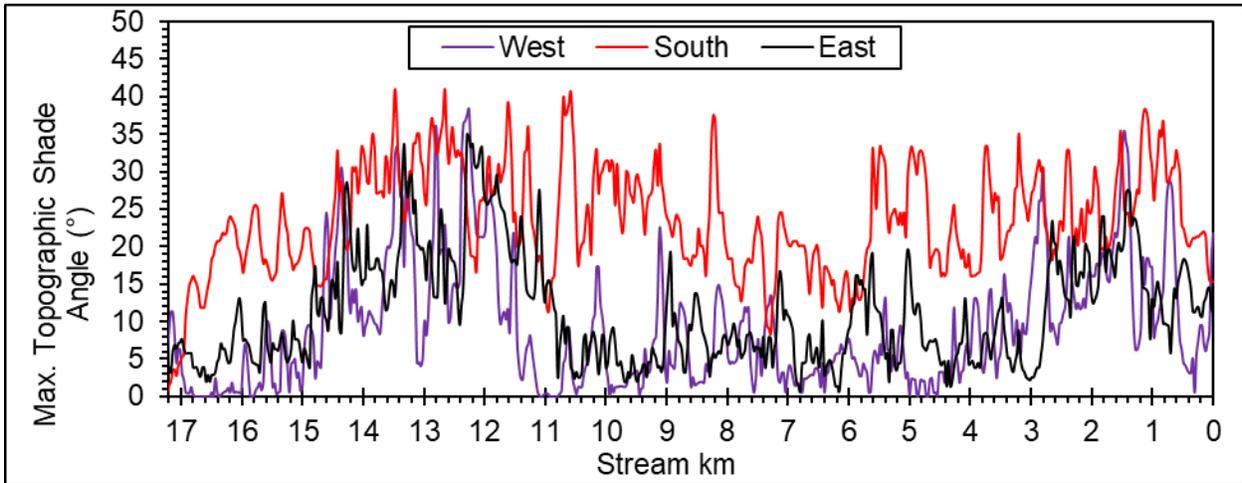
Figure 3-24: Little Sandy River model inputs: Maximum topographic shade angles.
