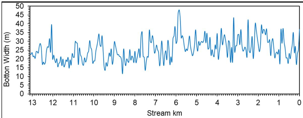
Figure 3-12: Salmon River model inputs: Bottom width.
