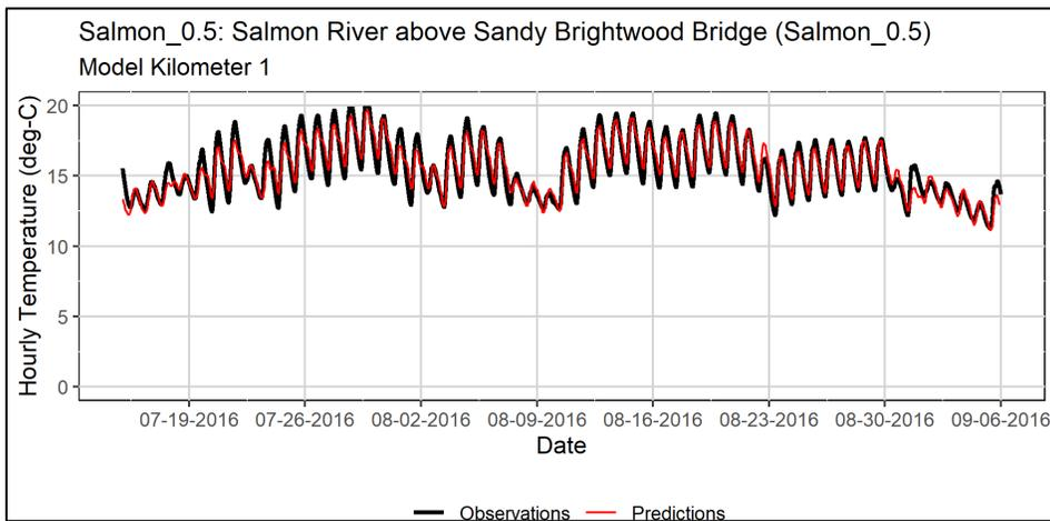
Figure 3-15: Salmon River above Sandy Brightwood Bridge: Modeled vs. observed hourly temperatures.
