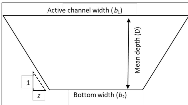
Figure 2-3: Equation 2-1 conceptual diagram: Trapezoidal channel and terms.
