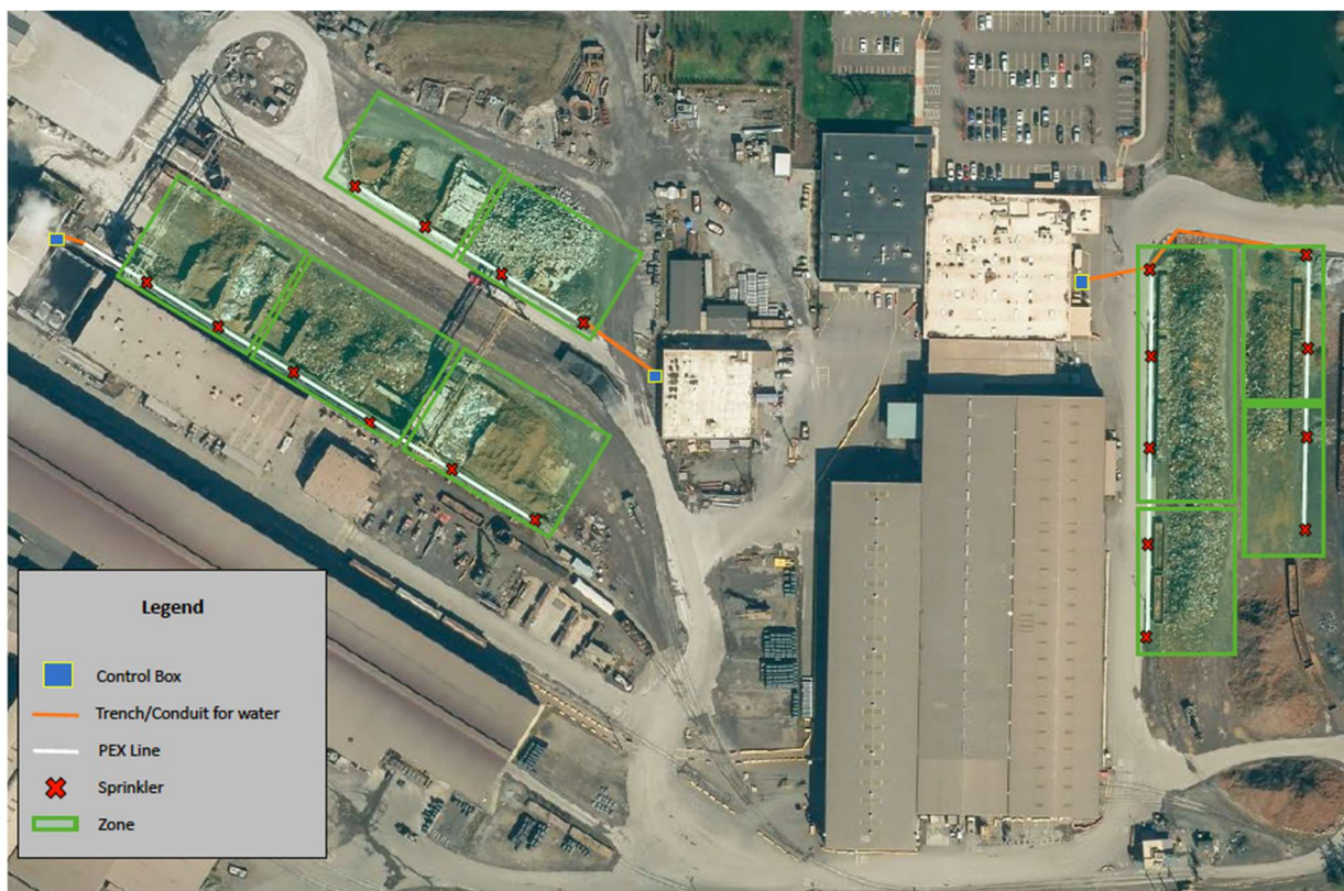
Figure 1 – Location of Water Spray System
