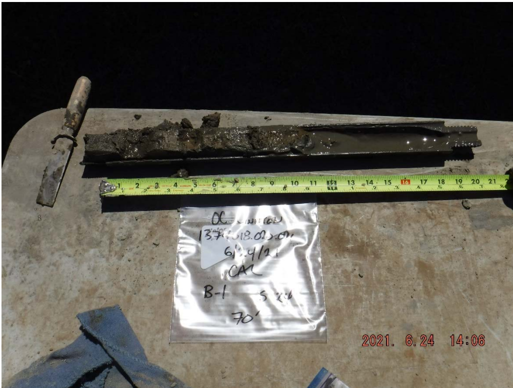
19. Boring B-1 at 70 feet: Gray-brown, very silty, fine to medium SAND.
