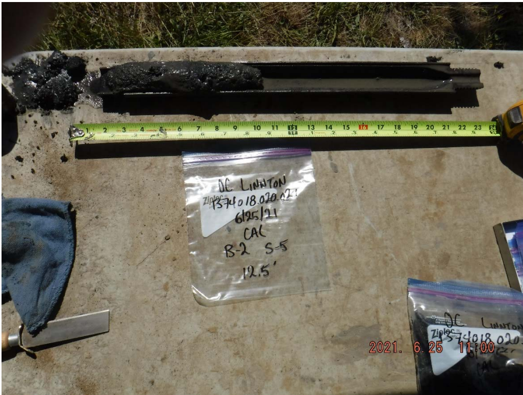
28. Boring B-2 at 12.5 feet: Dark gray to gray, fine to coarse SAND with gravel and silt.
