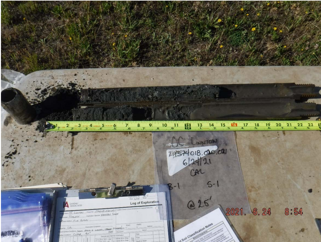
1. Boring B-1 at 2.5 feet: Dark gray, fine to coarse SAND with silt.
