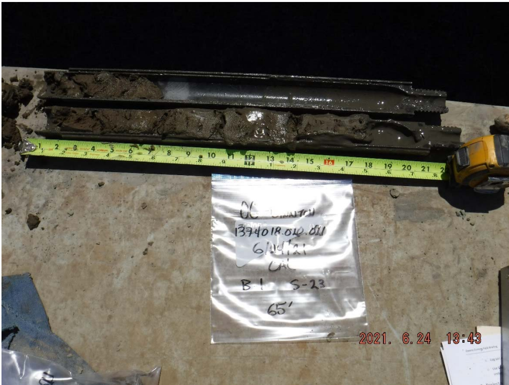
18. Boring B-1 at 65 feet: Gray-brown to brown SILT.
