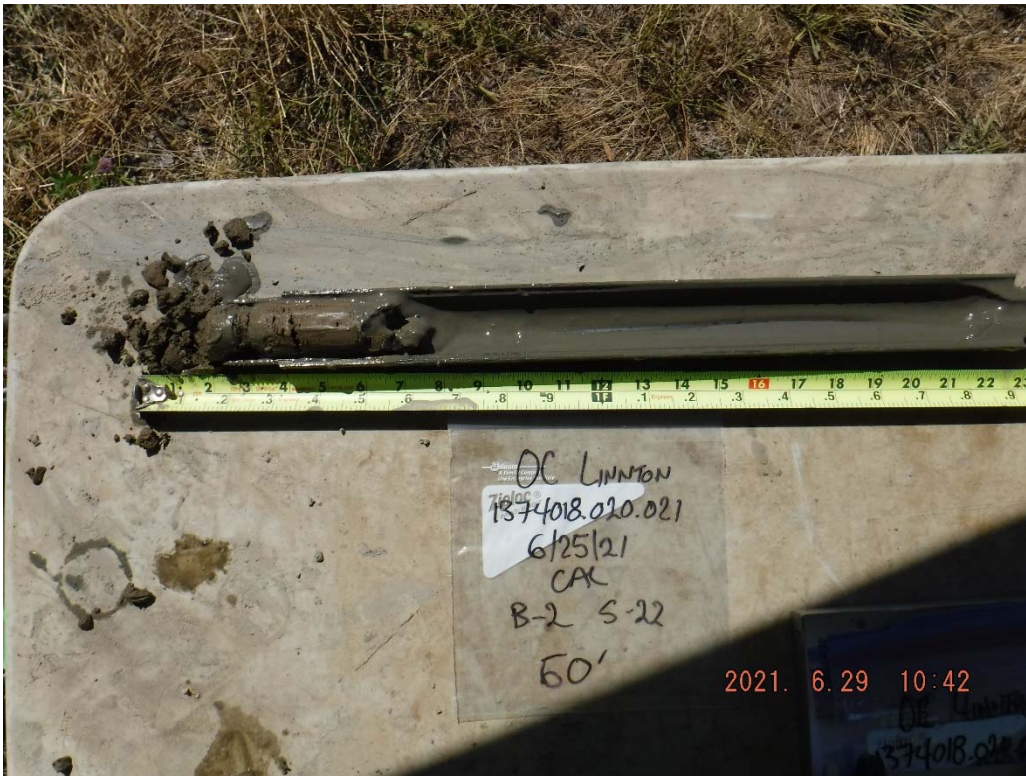
43. Boring B-2 at 60 feet: Gray-brown to brown SILT.
