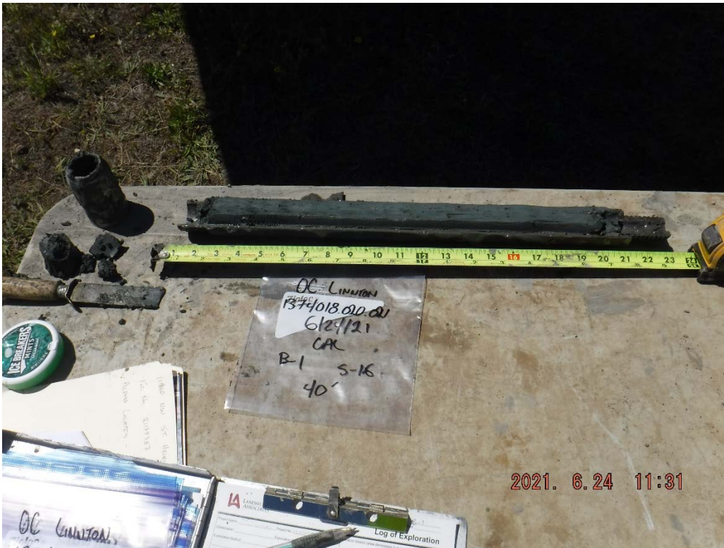
12. Boring B-1 at 40 feet: Blue-gray to gray SILT.
