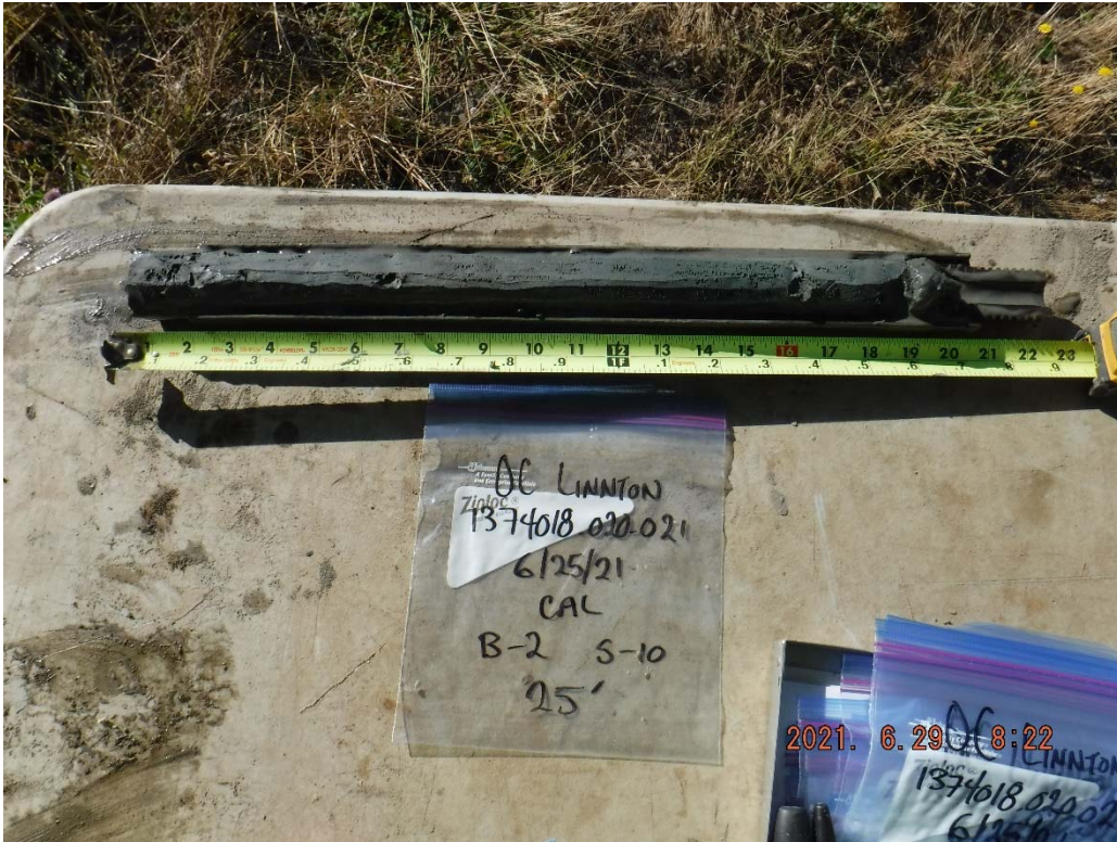
32. Boring B-2 at 25 feet: Gray, elastic SILT.
