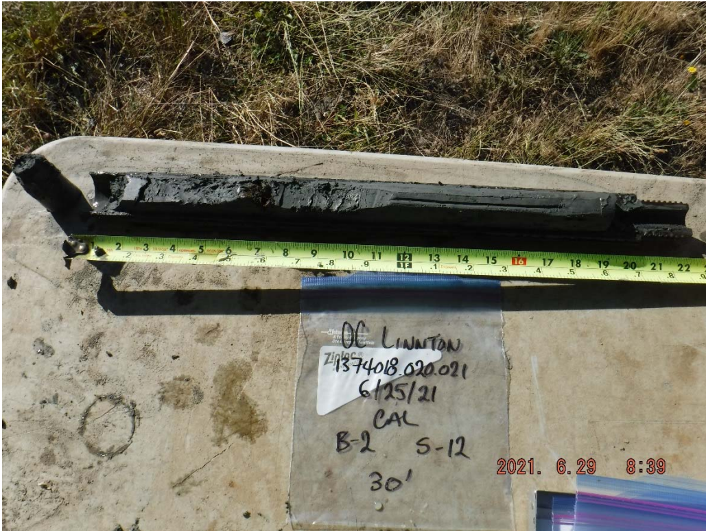
34. Boring B-2 at 30 feet: Dark gray SILT with trace organics.
