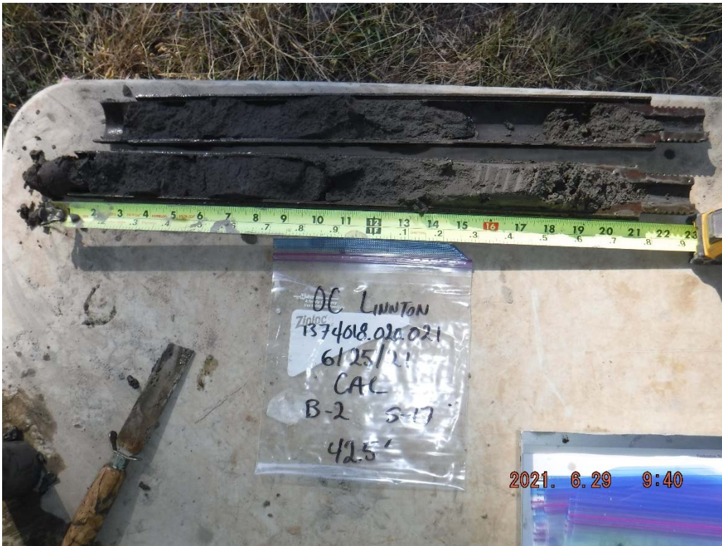
38. Boring B-2 at 42.5 feet: Dark gray SILT with trace organics.
