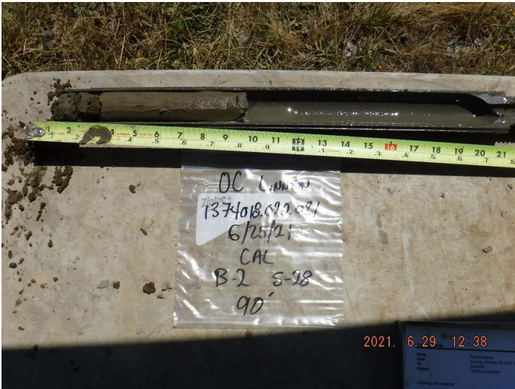
49. Boring B-2 at 90 feet: Gray-brown, very silty, fine SAND.
