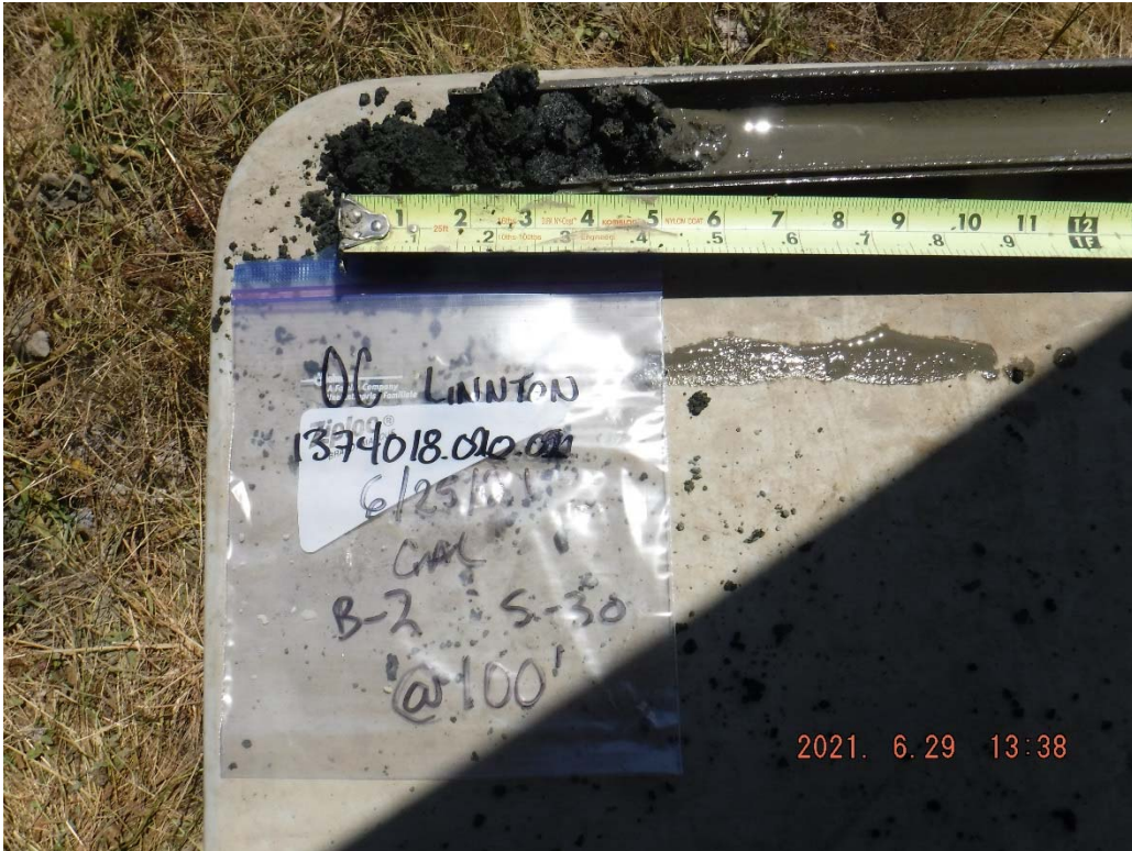
51. Boring B-2 at 100 feet: Basalt.
