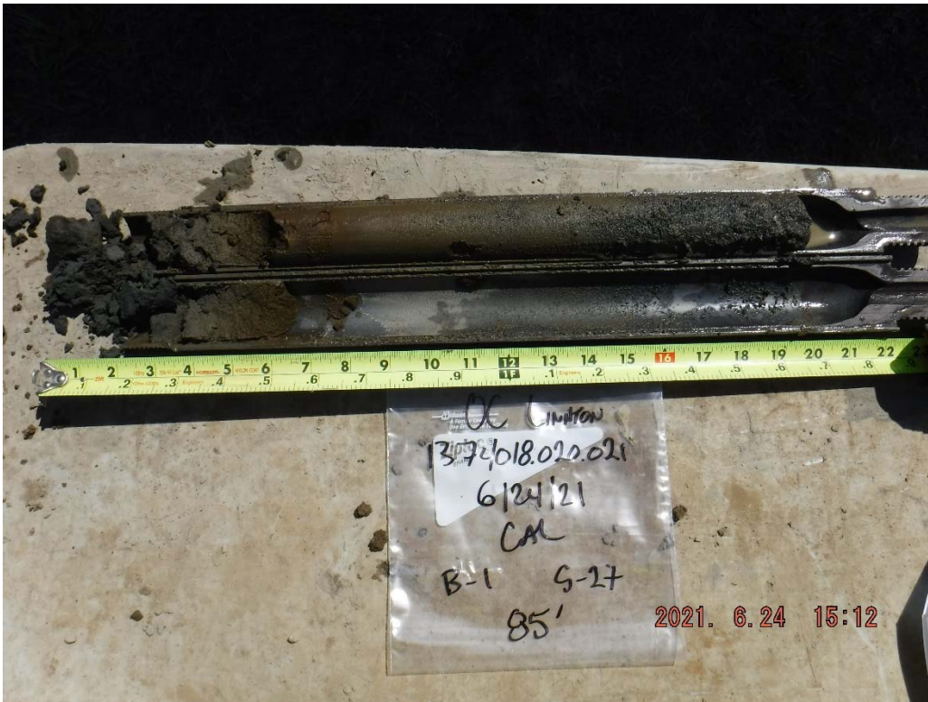
22. Boring B-1 at 85 feet: Brown, very silty, fine to medium SAND.
