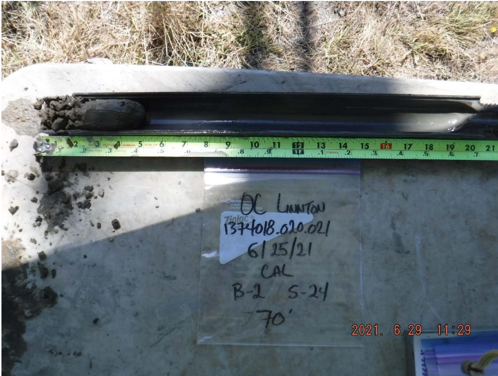
45. Boring B-2 at 70 feet: Gray, very sandy SILT with organics.
