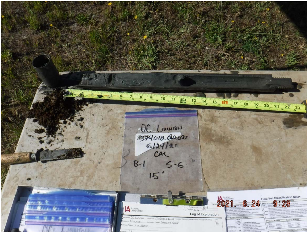
5. Boring B-1 at 15 feet: Dark gray, fine to coarse SAND with silt.
