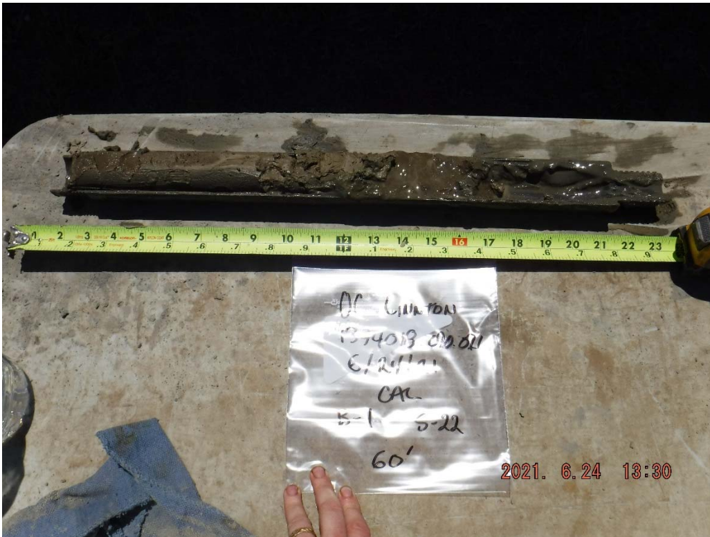
17. Boring B-1 at 60 feet: Gray-brown to brown SILT.
