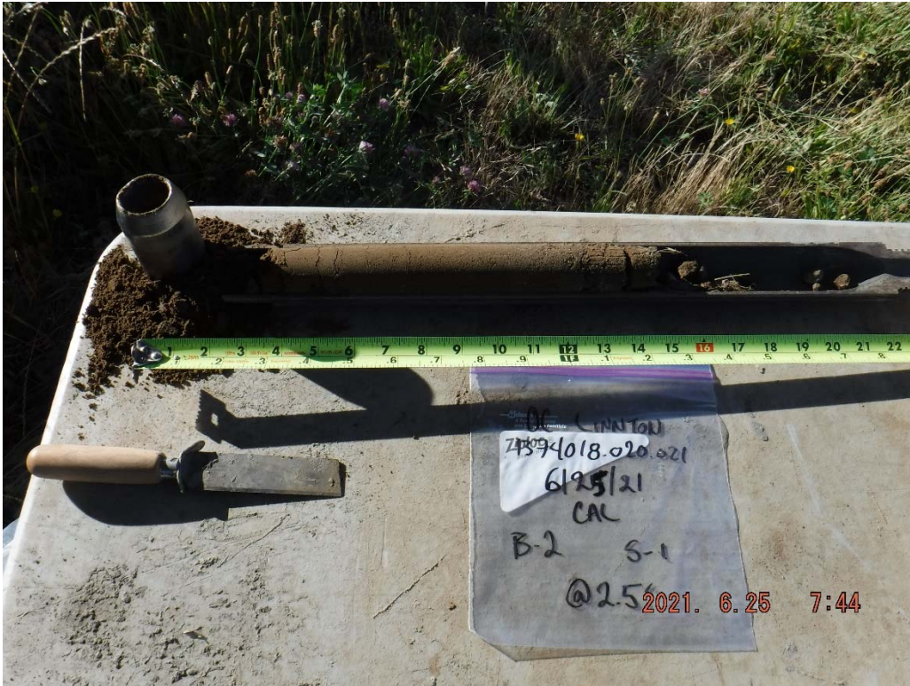
24. Boring B-2 at 2.5 feet: Brown, fine to coarse SAND.
