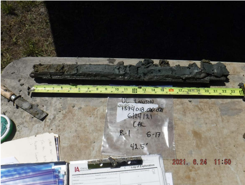
13. Boring B-1 at 42.5 feet: Gray-brown to gray CLAY.
