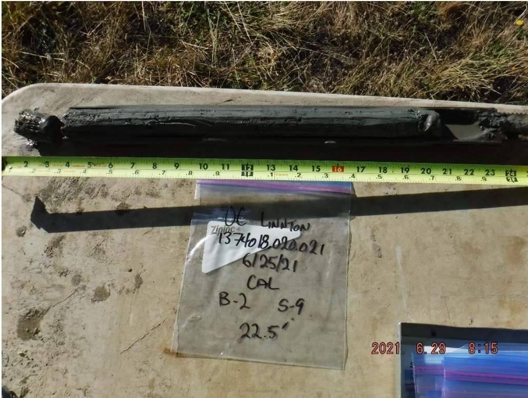
31. Boring B-2 at 22.5 feet: Light gray to gray, elastic SILT with organics.
