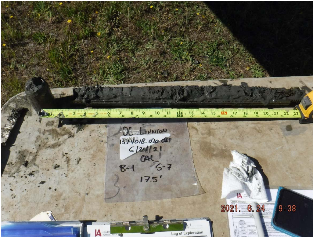
6. Boring B-1 at 17.5 feet: Gray SILT with wood debris.
