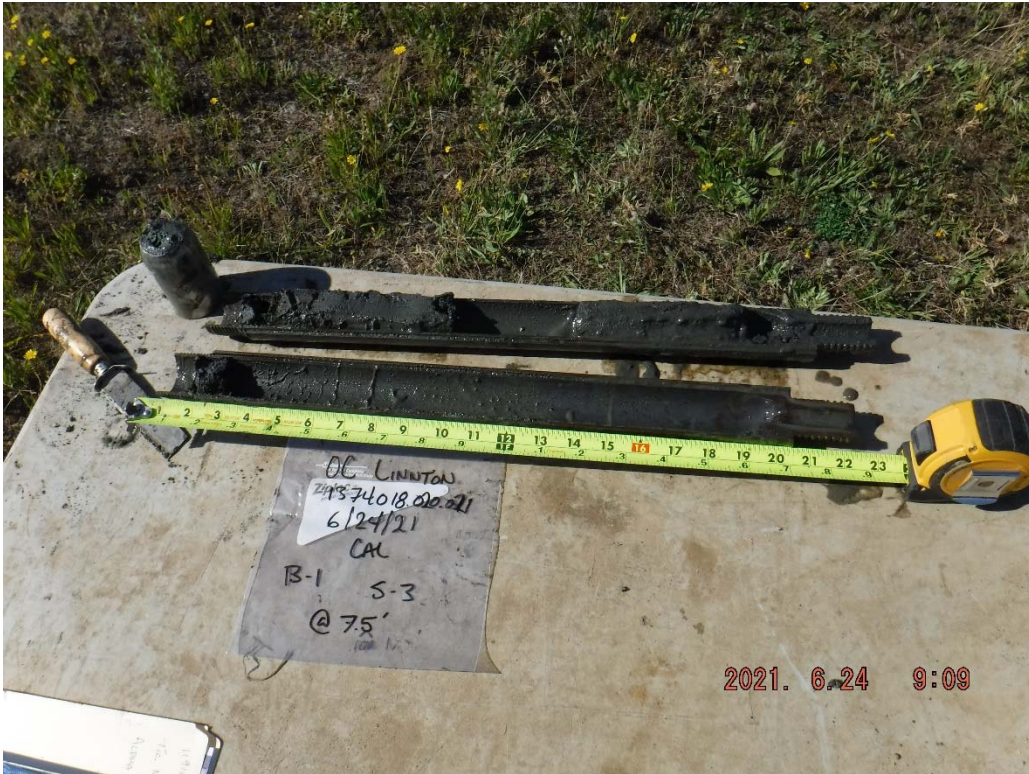
3. Boring B-1 at 7.5 feet: Gray SILT.
