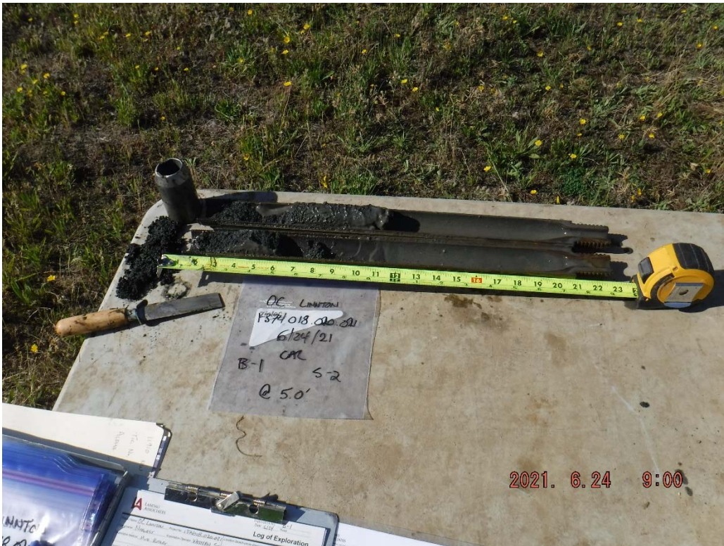
2. Boring B-1 at 5 feet: Dark gray, fine to coarse SAND with silt.
