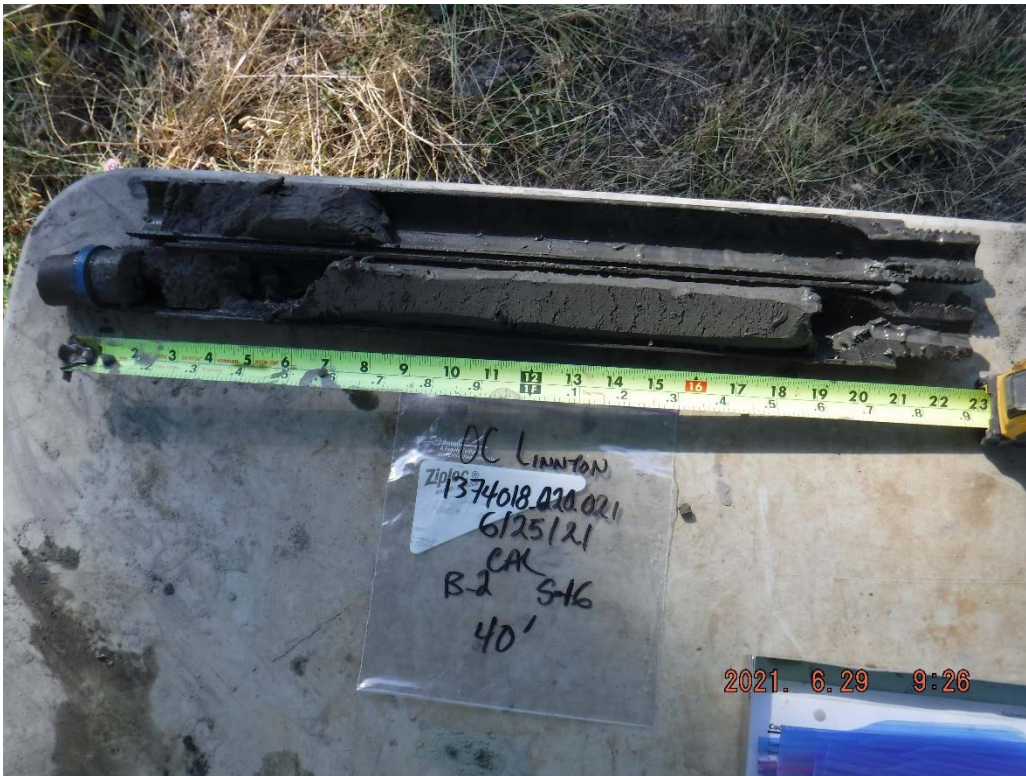
37. Boring B-2 at 40 feet: Dark gray SILT with trace organics.
