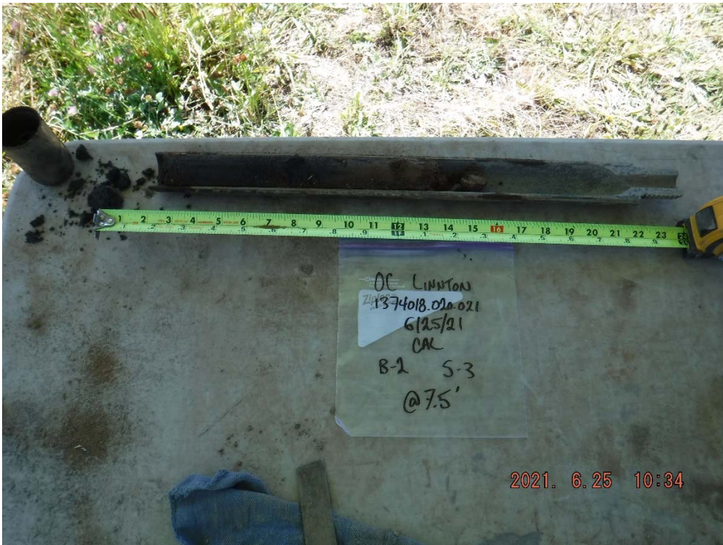
26. Boring B-2 at 7.5 feet: Light brown, silty, fine to coarse SAND with organics.
