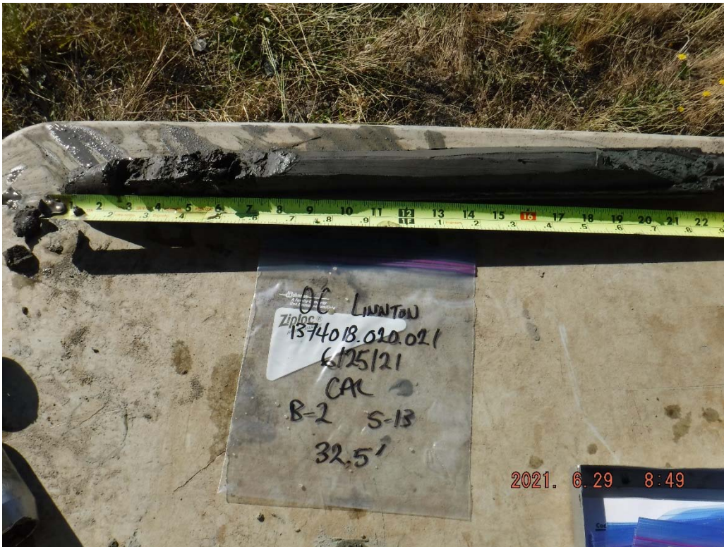
35. Boring B-2 at 32.5 feet: Dark gray SILT with trace organics.
