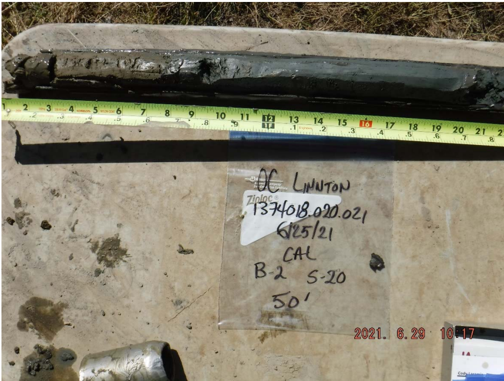
41. Boring B-2 at 50 feet: Gray to gray-brown SILT.
