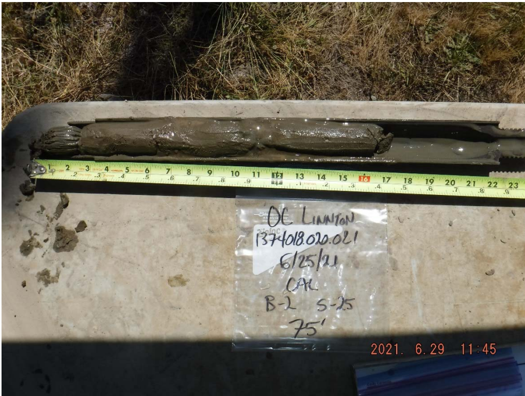
46. Boring B-2 at 75 feet: Gray-brown, sandy SILT with organics.
