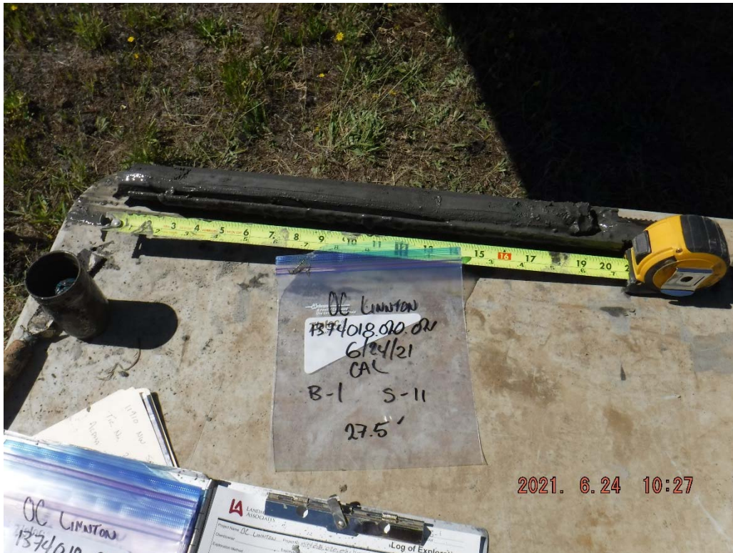
9. Boring B-1 at 27.5 feet: Dark gray SILT.
