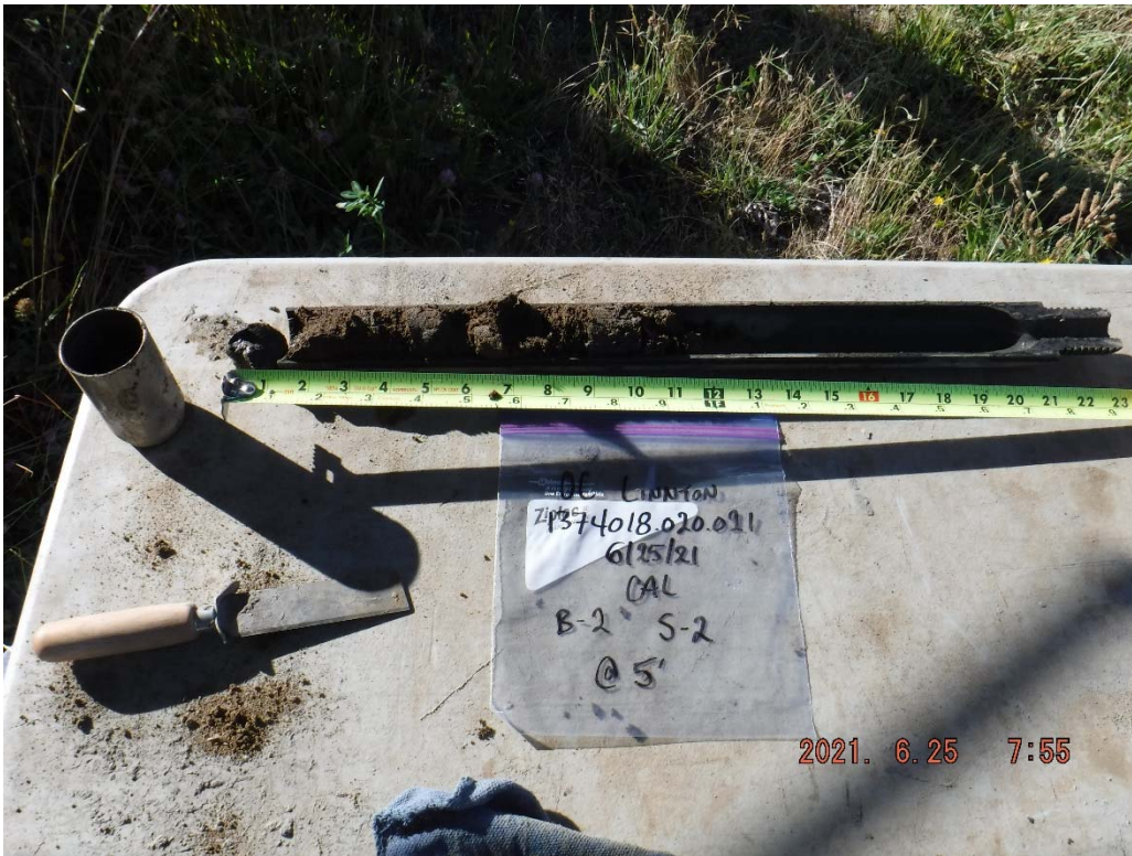
25. Boring B-2 at 5 feet: Brown, fine to coarse SAND.
