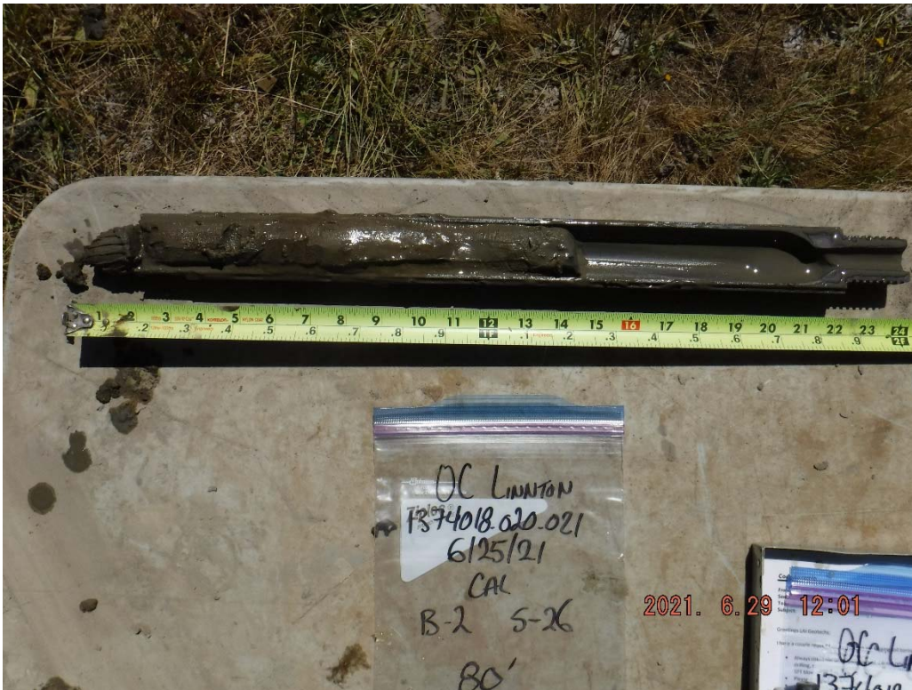
47. Boring B-2 at 80 feet: Gray-brown, very silty, fine SAND.
