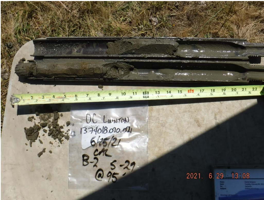
50. Boring B-2 at 95 feet: Gray-brown, fine SAND with silt.
