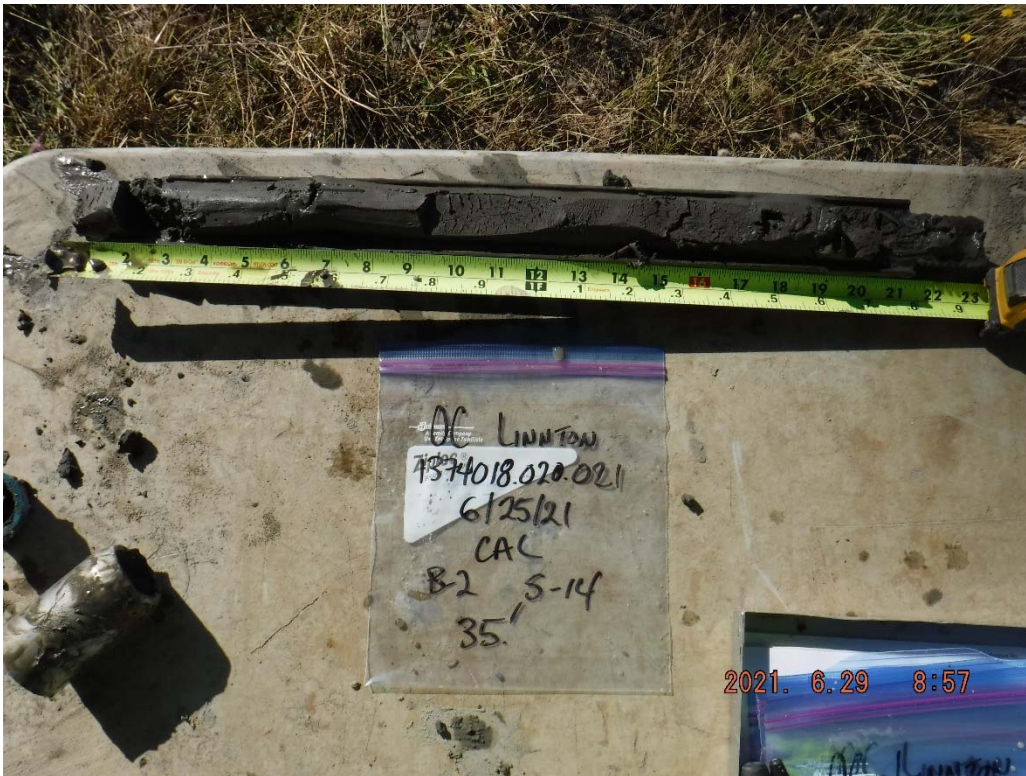
36. Boring B-2 at 35 feet: Dark gray SILT with trace organics.
