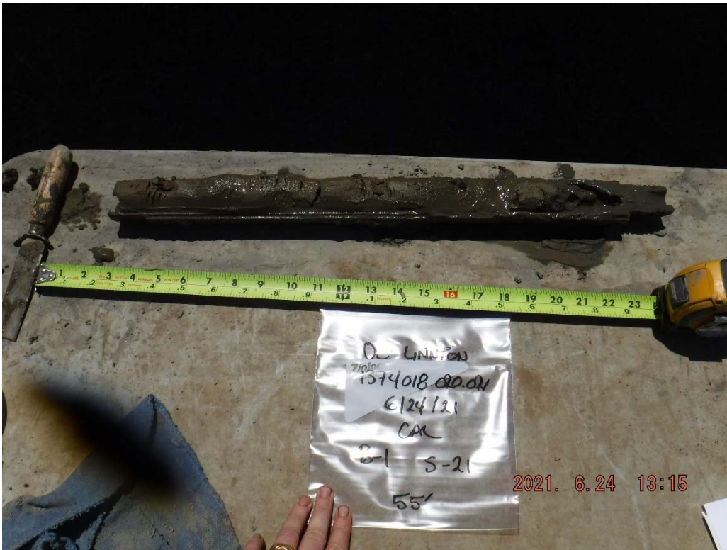
16. Boring B-1 at 55 feet: Gray-brown to brown SILT with fine sand.
