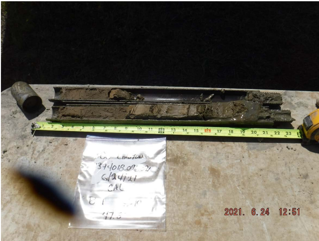
14. Boring B-1 at 47.5 feet: Gray-brown SILT and gray-brown, silty, fine to coarse SAND.
