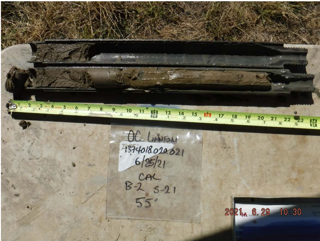
42. Boring B-2 at 55 feet: Gray-brown to brown SILT.
