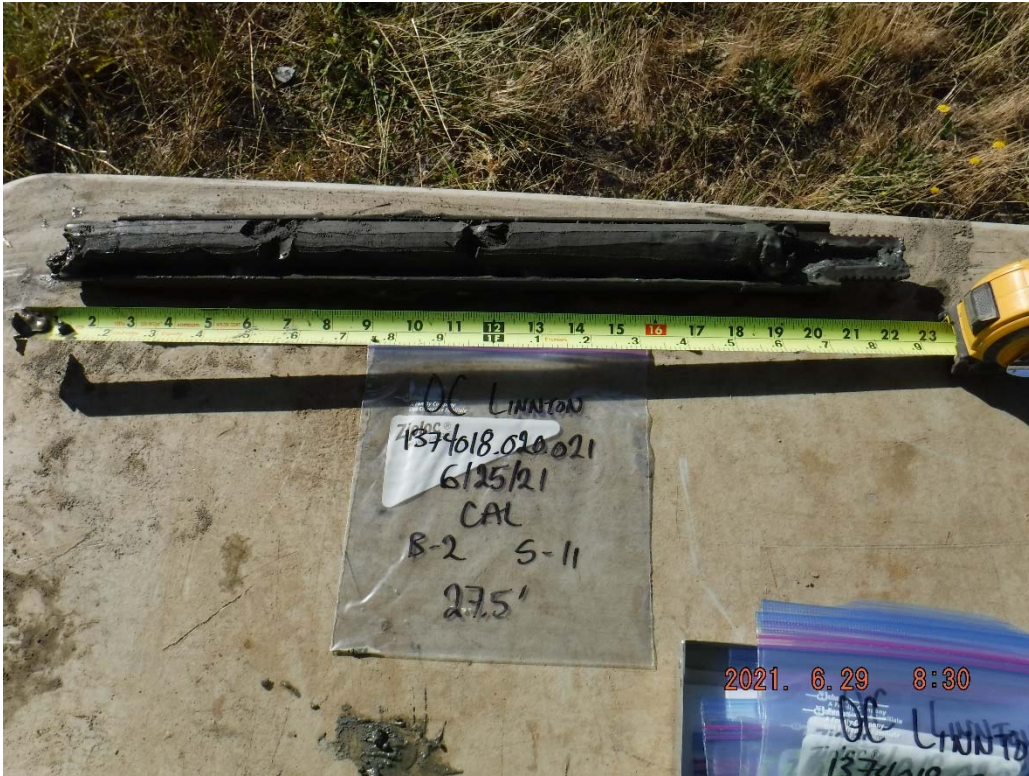
33. Boring B-2 at 27.5 feet: Dark gray SILT.
