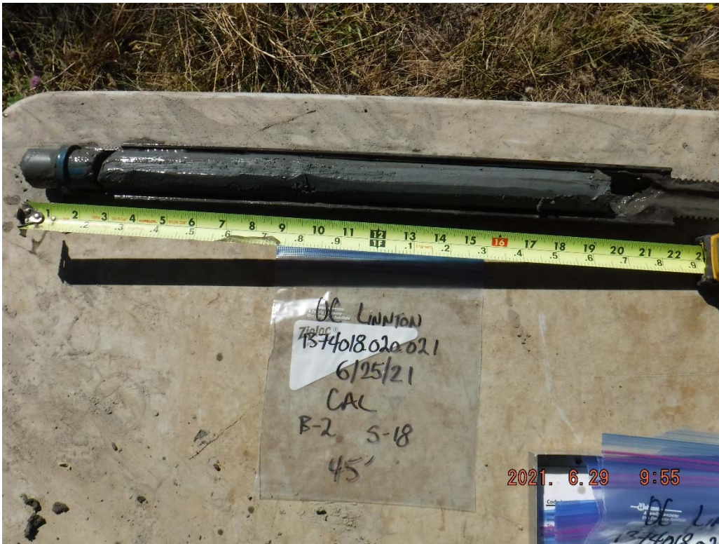
39. Boring B-2 at 45 feet: Light gray to blue-gray SILT with slickensides.
