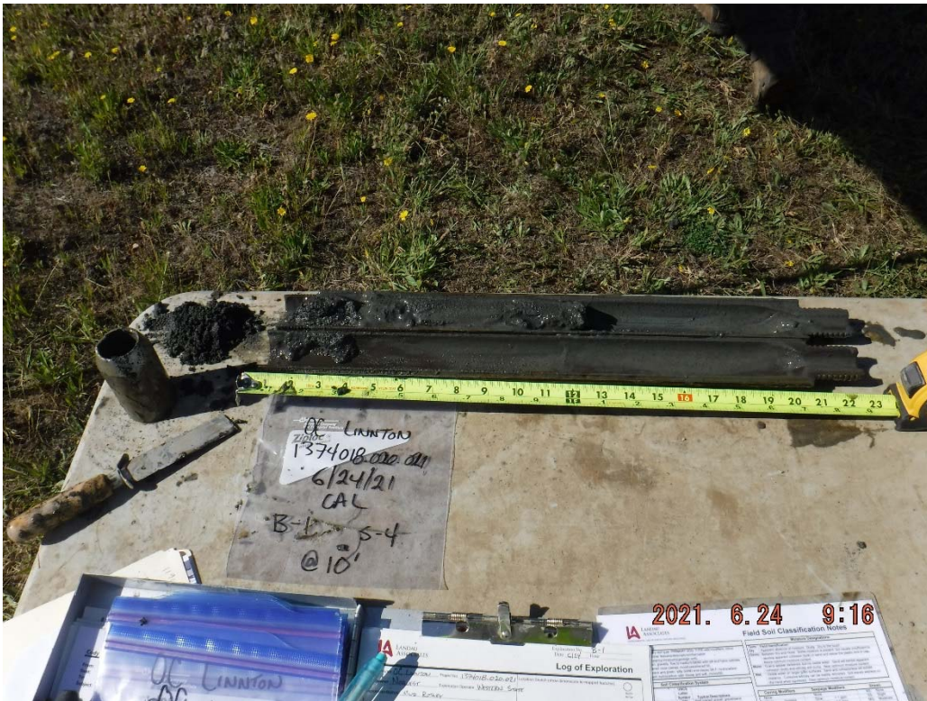
4. Boring B-1 at 10 feet: Dark gray, fine to coarse SAND with silt.
