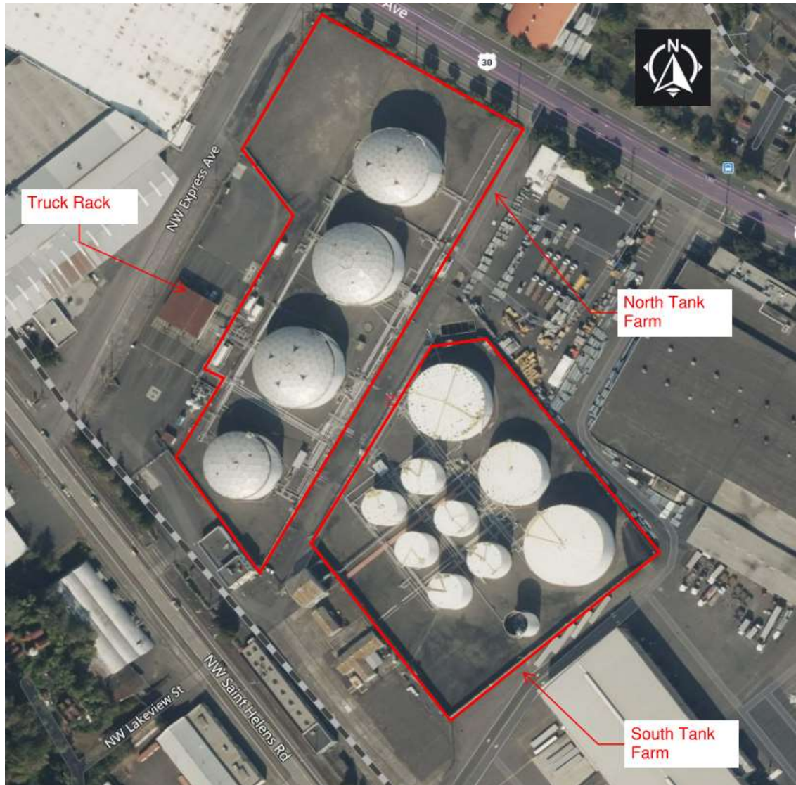
Figure 2-2: Aerial Plan of Shell Portland Terminal
