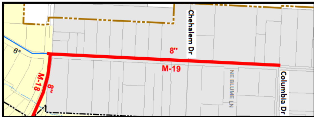
FIGURE 4 CHEHALEM DRIVE PUBLIC WATER SERVICE LINE EXTENSION
