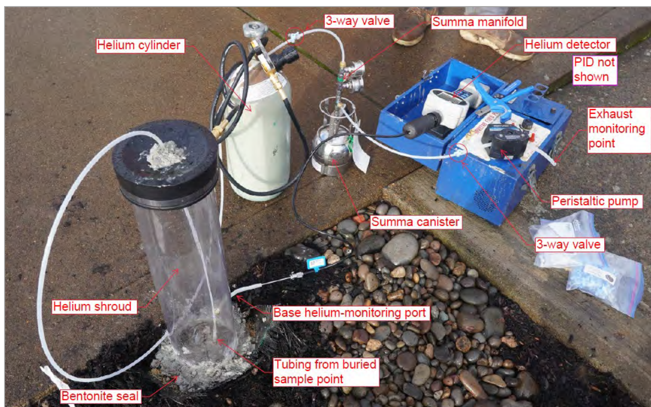
Exhibit 1. Soil vapor sampling set-up.
