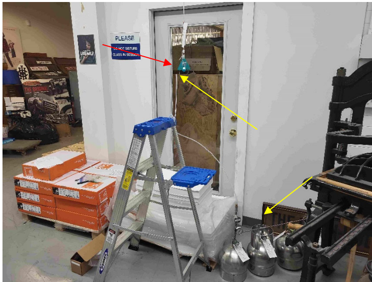
Radiello passive sampler (red) and TO-15 Summa canisters (yellow) with extended inlet deployed concurrently to monitor indoor air
