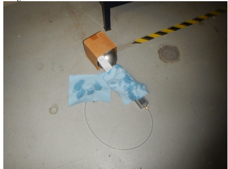
Sampling sub-slab vapor location SUB13 (NE part of NW quad). Note blue rags saturated with isopropyl alcohol for leak detection. (Typical)
