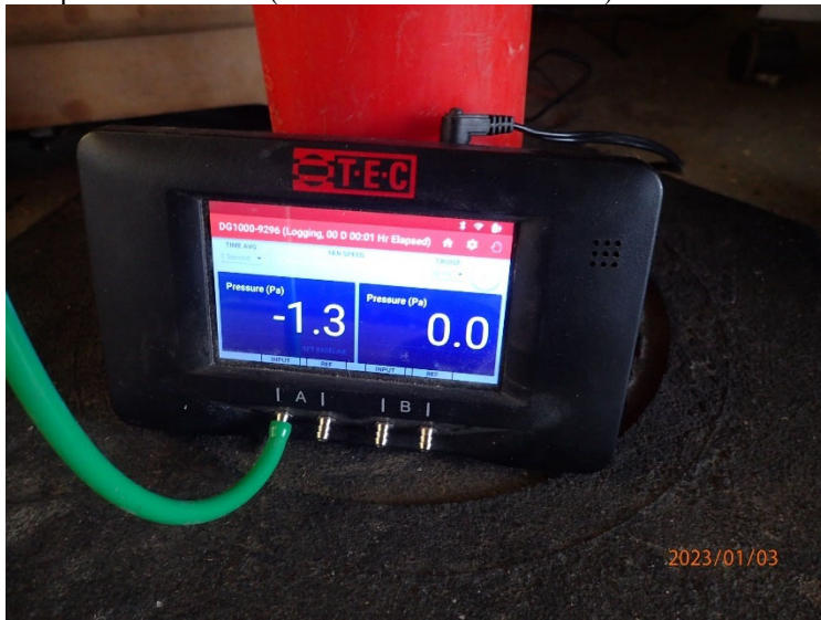
Differential pressure in units of Pascals (pa) were recorded at 5 second intervals.
