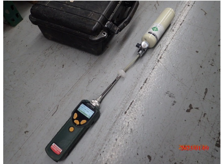
PID was calibrated prior to being used to monitoring sub-slab vapor / soil gas.
