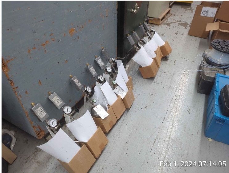
Checking flow controller ID and Summa canister ID prior to sampling.
