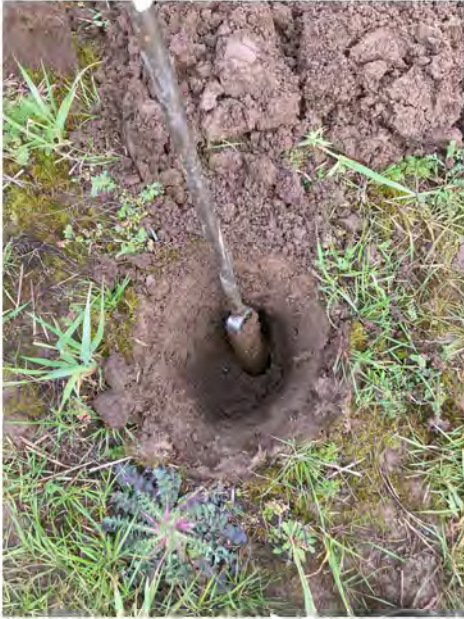
Photo 13 - View of a hand auger sample being collected at sample location C13. (2/21/2024)
