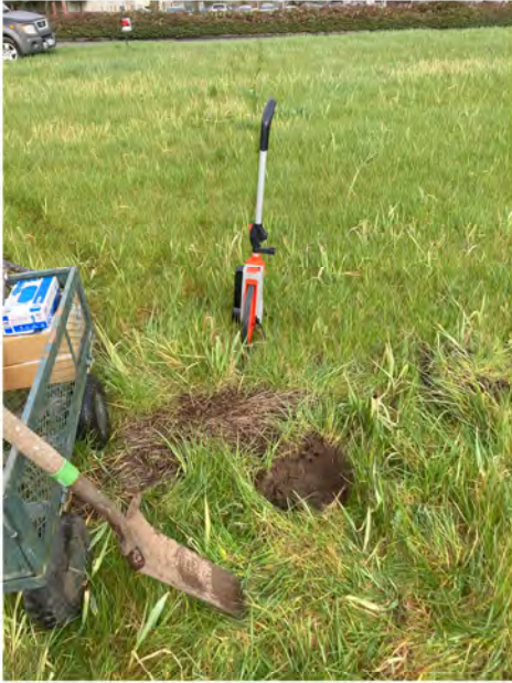
Photo 9 - View of follow-up soil sampling activities at sample location C1, looking north. A 1-foot hole was 1st dug with a shovel. (2/21/2024)
