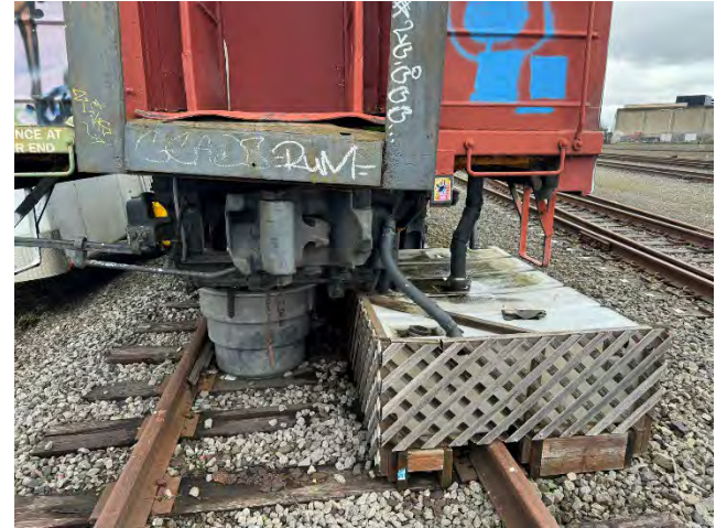
Sewage collection at the rail cars.
