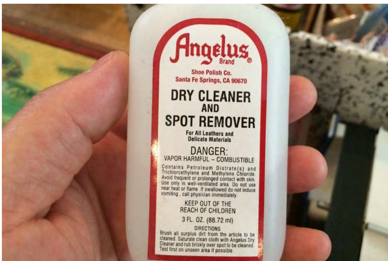
Photograph 22 – One of the cleaning supplies stored under the countertop in the first floor space. This contains specifically TCE which was detected at a relatively high concentration in July 2015.
