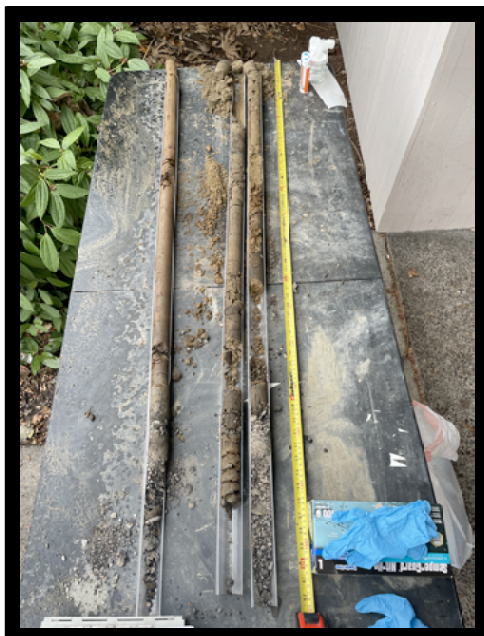
Photograph 9: Soil cores from borings P8 and P9. The top of the soil cores are at the bottom of the photo. The cores for P8 are on the right side of the photograph, and the first core (0 to 5 ft bgs) is the furthest right. The core for boring P9 is on the left side of the photograph.
