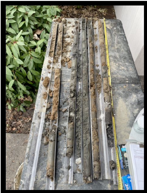
Photograph 14: Soil cores from boring P12. The top of the soil cores are at the bottom of the photo, and the first core (0 to 5 ft bgs) is on the right side of the photograph. The deepest core (20 ft to 25 ft bgs) is on the left side of the photograph.
