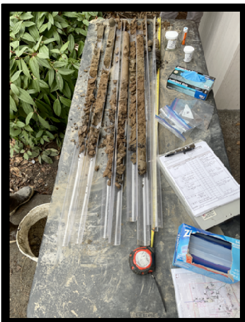
Photograph 15: Soil cores from boring P13. The top of the soil cores are at the bottom of the photo, and the first core (0 to 5 ft bgs) is on the right side of the photograph. The deepest core (15 ft to 20 ft bgs) is on the left side of the photograph.
