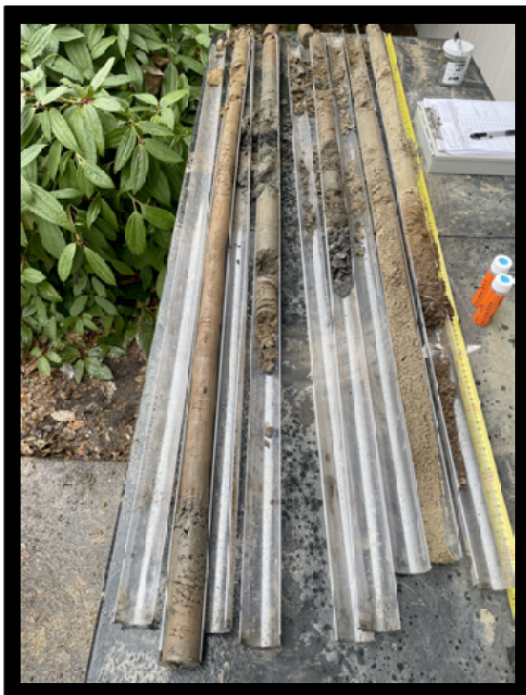
Photograph 13: Soil cores from borings P10 and P13. The top of the soil cores are at the bottom of the photo, and the two cores on the right side of the photograph are for boring P10. The cores for boring P13 are the three from the left of the photograph, with the shallow core (0 ft to 5 ft bgs) in the center, and the deepest core (10 ft to 15 ft bgs) on the left side of the photograph.
