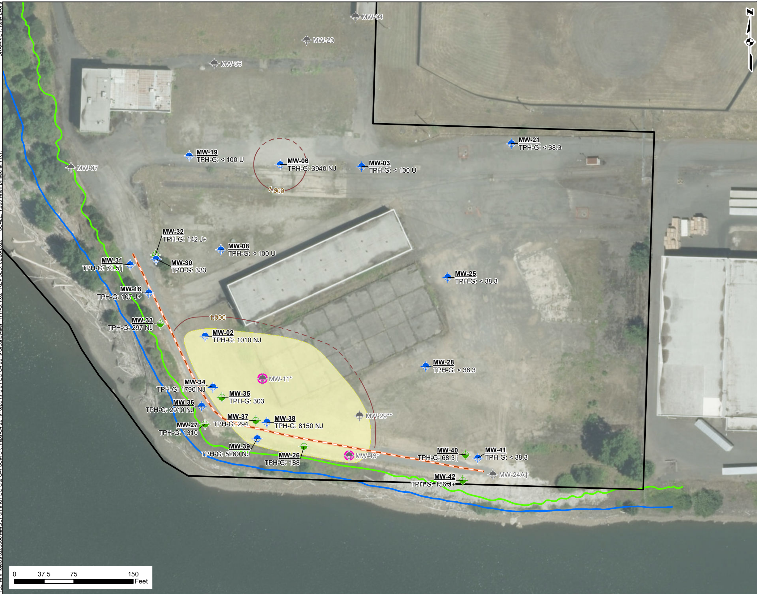
Figure 8 TPH-Gx Concentrations in Groundwater Q4 Performance Monitoring Report Premier Edible Oils 10400 N Burgard Way Portland, Oregon Environmental Resources Management www.erm.com
