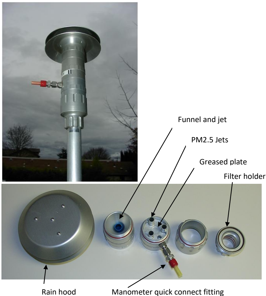
Figure 4. PM 2.5 Inlet with smart manometer connection.
