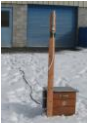
Figure 3. Survey Sampler (without inlet).
