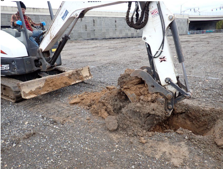
A small backhoe was used to facilitate the collection 50 increments of soil from DU01 through DU04.
