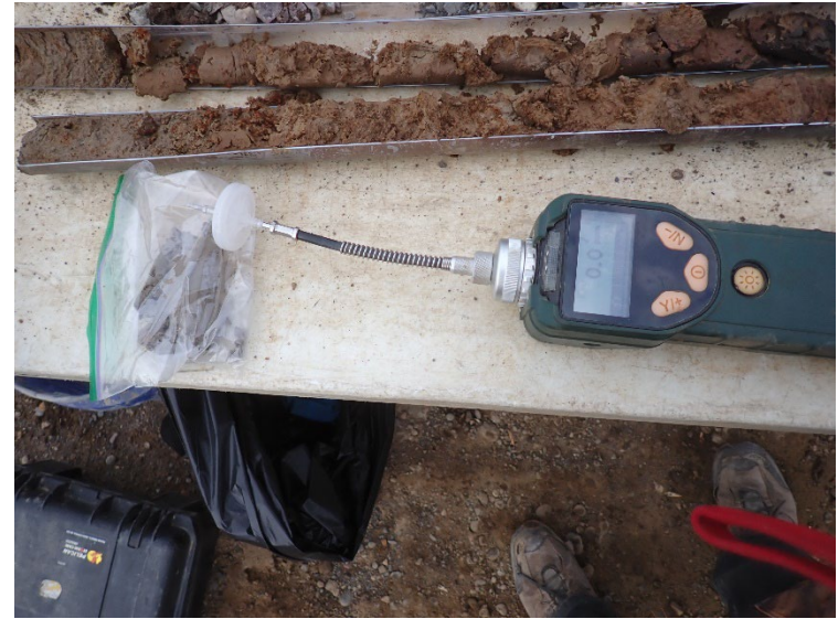
Soils were screened continuously for potential volatile using a PID.
