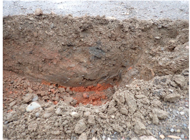
View of brick material encountered in soils beneath DU04.
