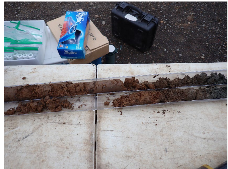
Soils encountered in borings were generally described as silts and sands extending to around 10 to 20 feet bgs.
