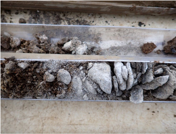
View of gravels encountered beneath the shallow, relatively fine-grained sediments.
