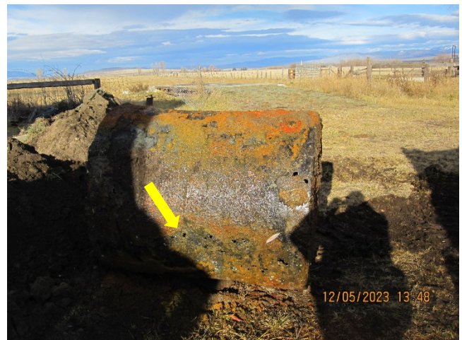
Photo 10: View of bottom of UST. Note numerous holes to right of arrow.
