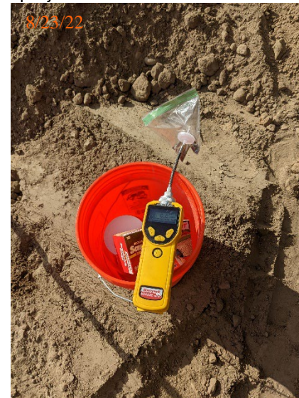
Soil increments were field screened for volatile organic constituents (VOCs) using a photoionization detector (PID).
