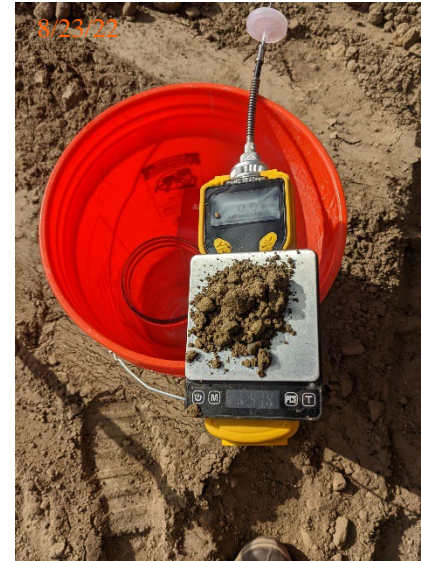
50 increments of approximately 40 grams each comprised one incremental sample. Increments were placed into a single one-gallon glass sample jar.
