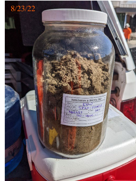
All 50 increments comprising incremental sample SP20-220823 were placed in a laboratory-prepared 1-gallon glass sample jar.
