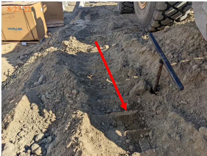
View of sample collection with stainless-steel hand auger. A de minimis area of darker soil was observed but there was no associated odor, or PID response.
