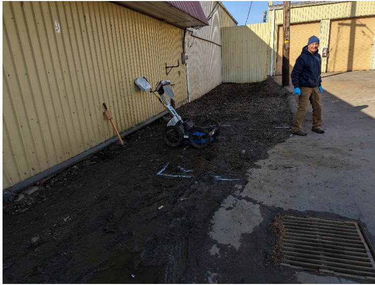
A geophysical survey was conducted to outline magnetic anomalies (MA02 on the north side of the building near the property margin).
