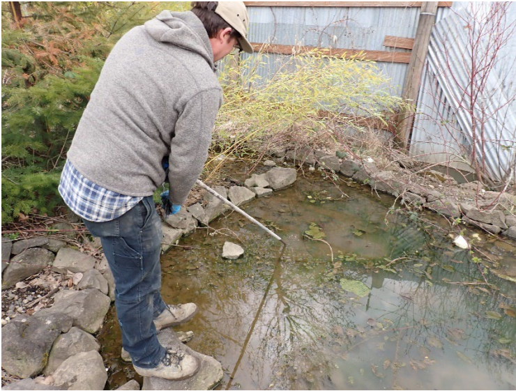
Pond (DU-2) sediments were sampled using a decontaminated stainless-steel hand auger.
