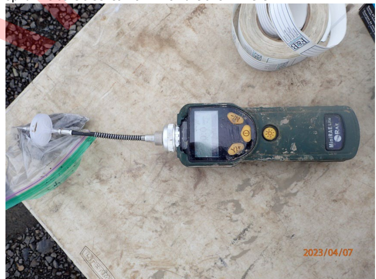
A photoionization detector (PID) was used to conduct field headspace screening for volatile organic constituents (VOCs).
