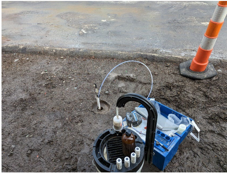
Reconnaissance ground water sampling using a peristaltic pump at EB01.
