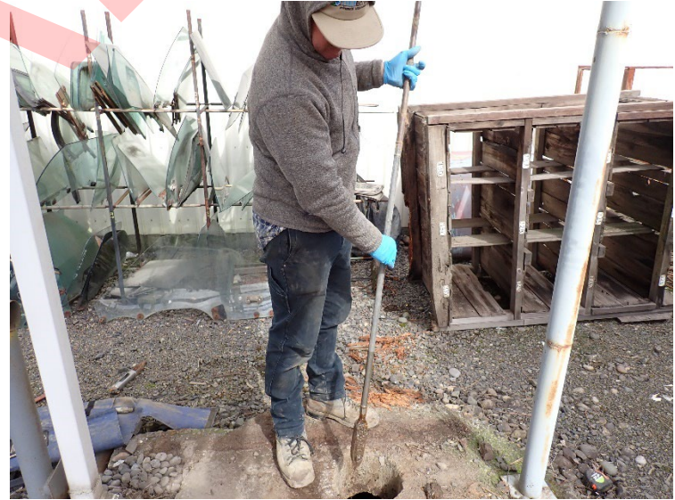
Using a stainless-steel hand auger to sample sediment within the UIC at the site.
