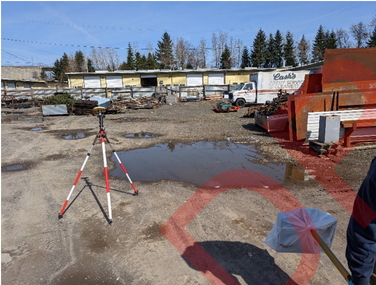
The locations of magnetic anomalies were recorded using a tripod-mounted GPS receiver.
