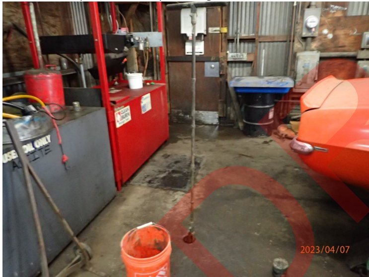
Soil samples were collected from EB07 using a decontaminated stainless-steel hand auger.
