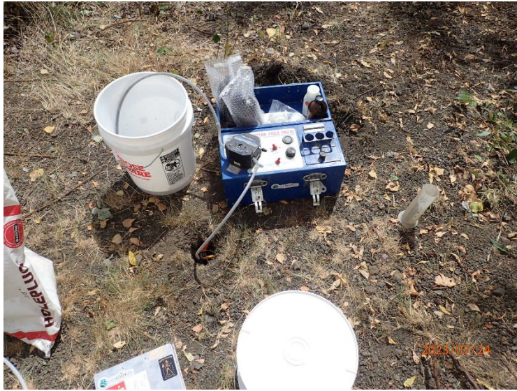
Reconnaissance ground water sample collection at B24 using a peristaltic pump.
