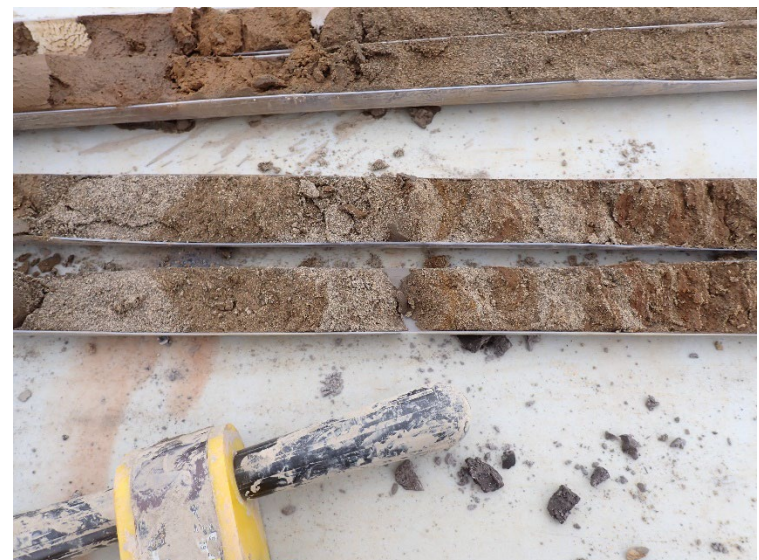
Brown and gray poorly graded sand underlain by poorly graded sand with silt in boring B21.
