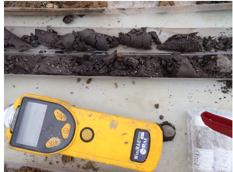
Field headspace volatiles screening of soil core using a photoionization detector (PID).
