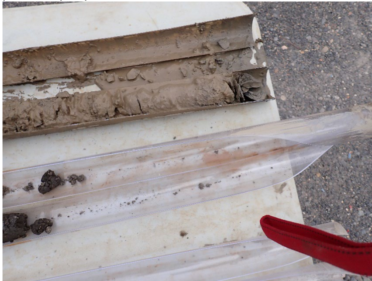
View of soil cores from boring B23 at the soil-water interface.
