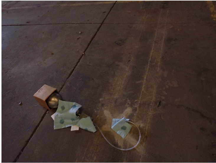
View of sub-slab vapor sampling using TO-15 equipment. Note the rags treated with isopropyl alcohol for leak detection.
