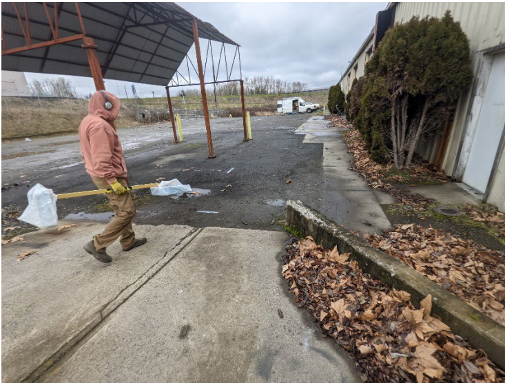
View of the geophysical survey using electromagnetic scanner.
