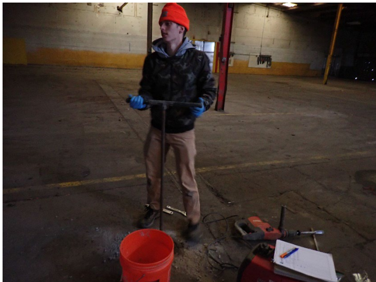
View of advancing a temporary soil boring indoors using a stainless-steel hand auger.
