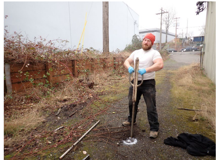
A slide hammer was utilized to set temporary soil gas sample probes.
