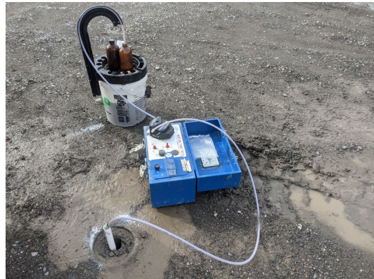
View of reconnaissance ground water sampling from temporary DPT boring.
