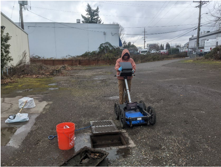
View of the geophysical survey using ground-penetrating radar.
