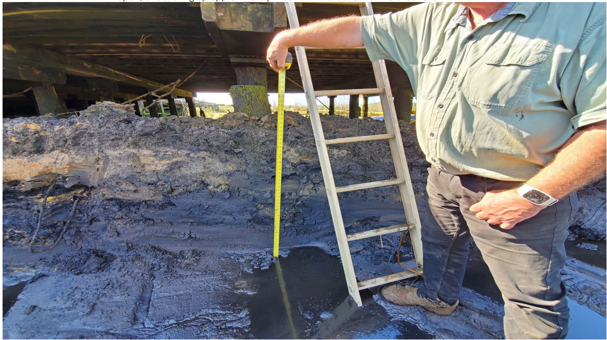
Photo 8: Depth of the southern dredged portion of MW#3, adjacent to walkway, measuring approximately 42 inches
