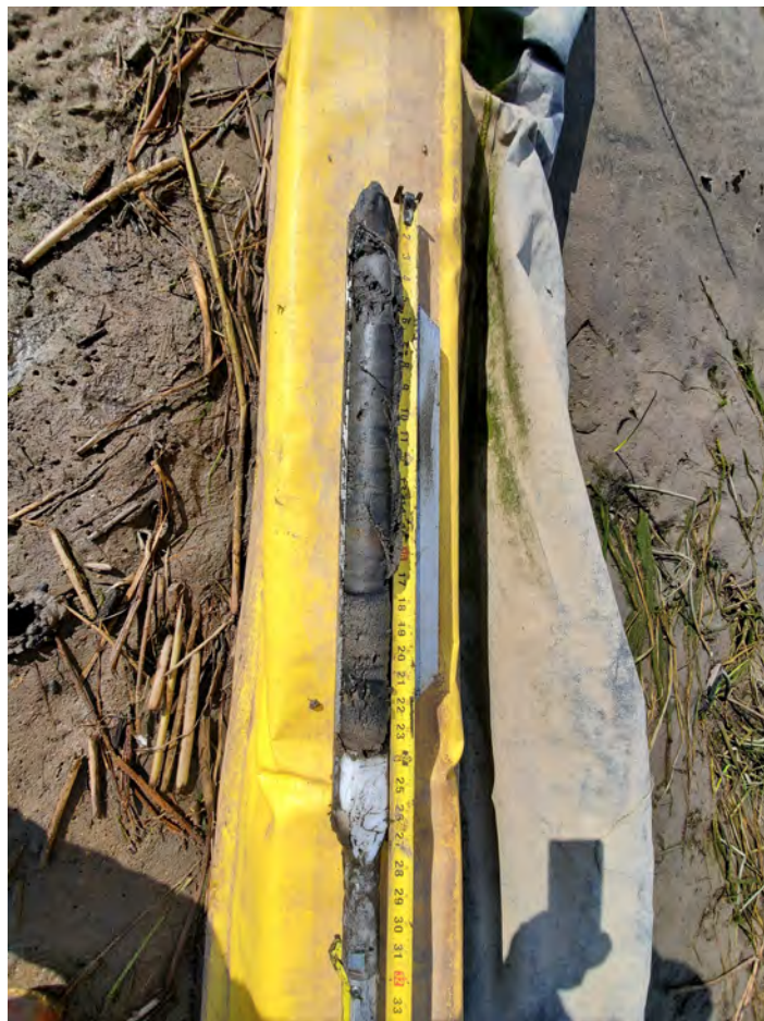
EMNR Sample 10: Photo showing a sand layer depth of 14".
