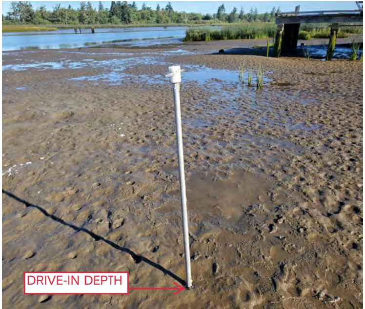
Photo 5: A look at the drive-in location of the russian pete bore at SP 12
