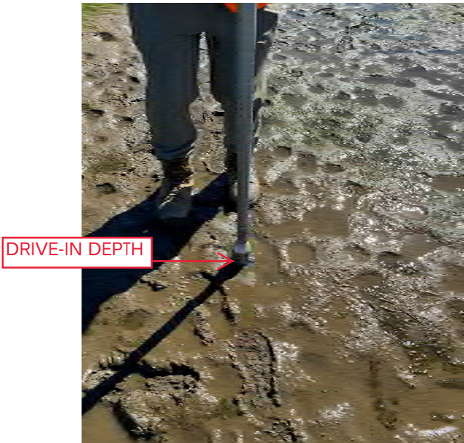
Photo 15: A look at the drive-in location of the russian pete bore at SP 21
