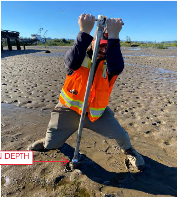
Photo 9: A look at the drive-in location of the russian pete bore at SP 14
