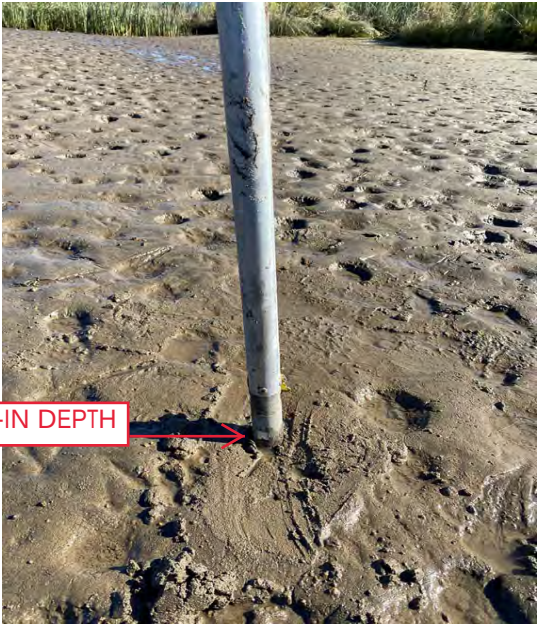
Photo 15: A look at the drive-in location of the russian pete bore at SP 18
