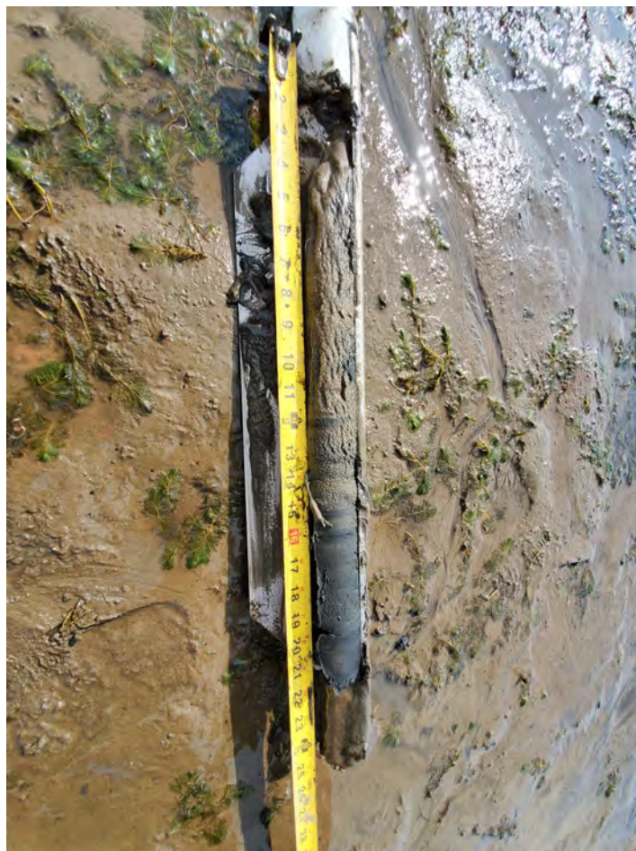
EMNR Sample 8: Photo showing a sand layer depth of 15".
