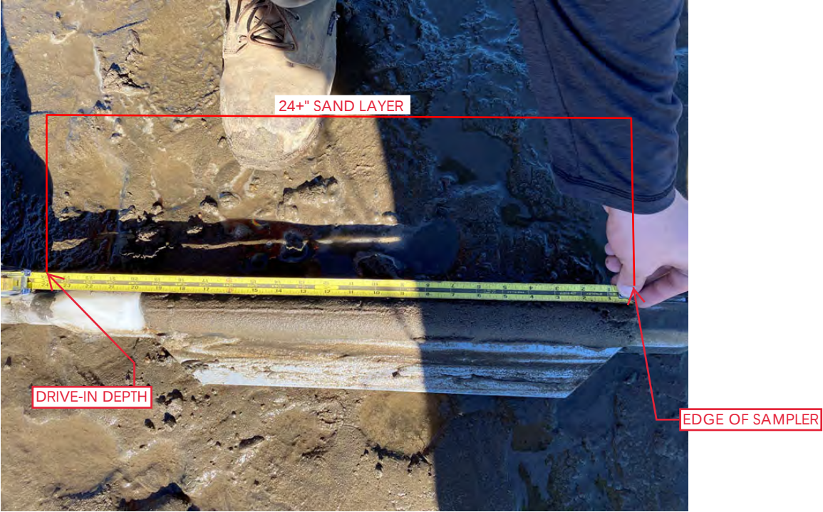
Photo 14: A look at the sampled EMNR Sand profile collected at SP 18, with a depth of over 24" (located within the transition/overlap zone near north dredge area prism)
