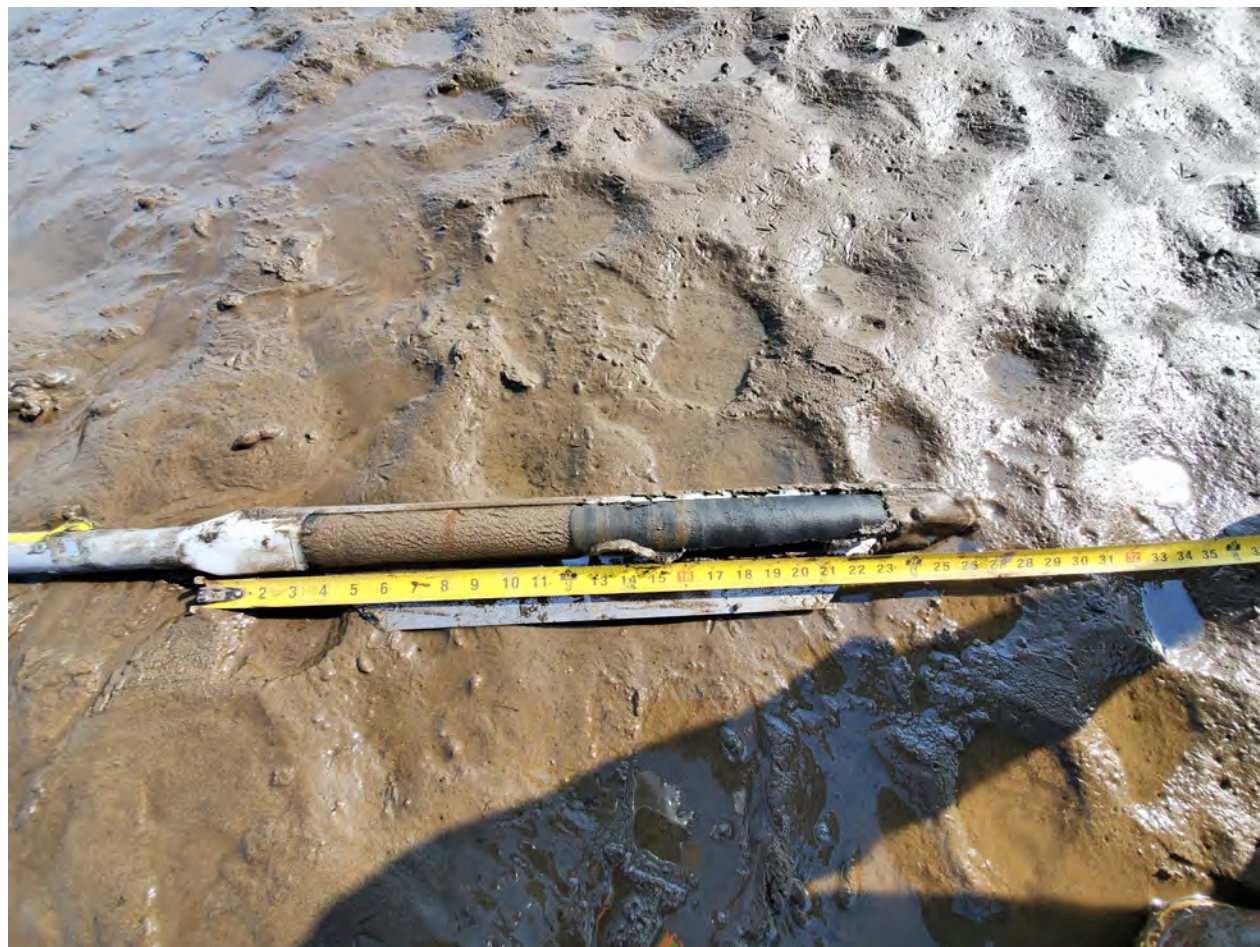
EMNR Sample 4: Photo showing a sand layer thickness of 12".
