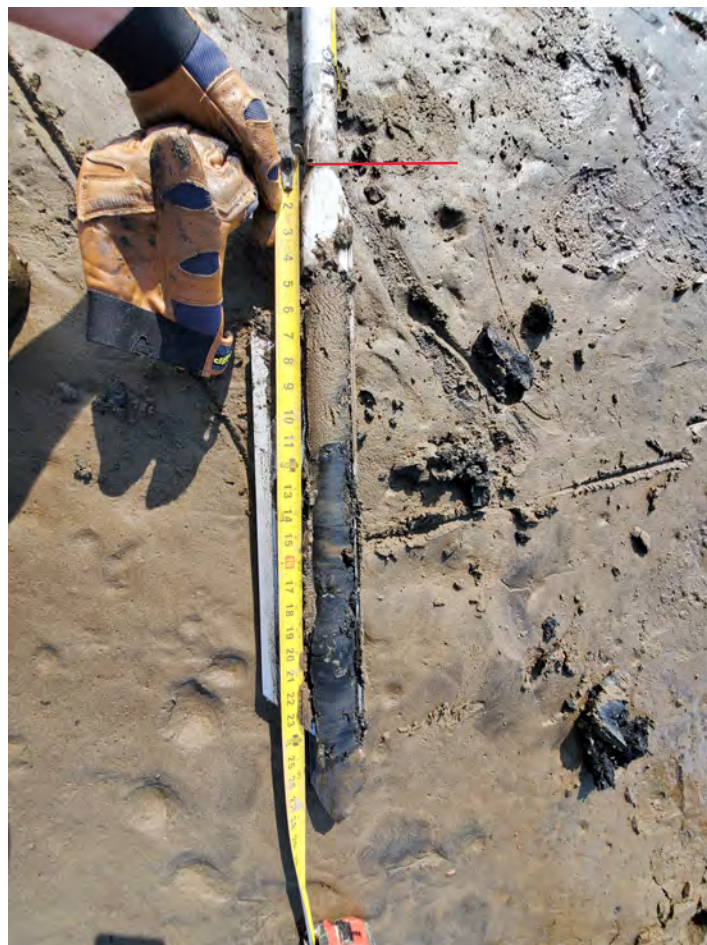
EMNR Sample 2: Photo showing a sand layer thickness of 11".
