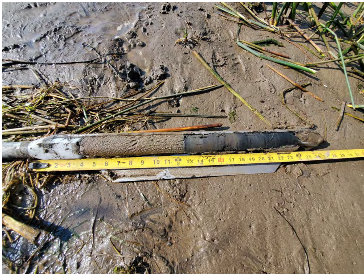
EMNR Sample 6: Photo showing a sand layer thickness of 12.5".
