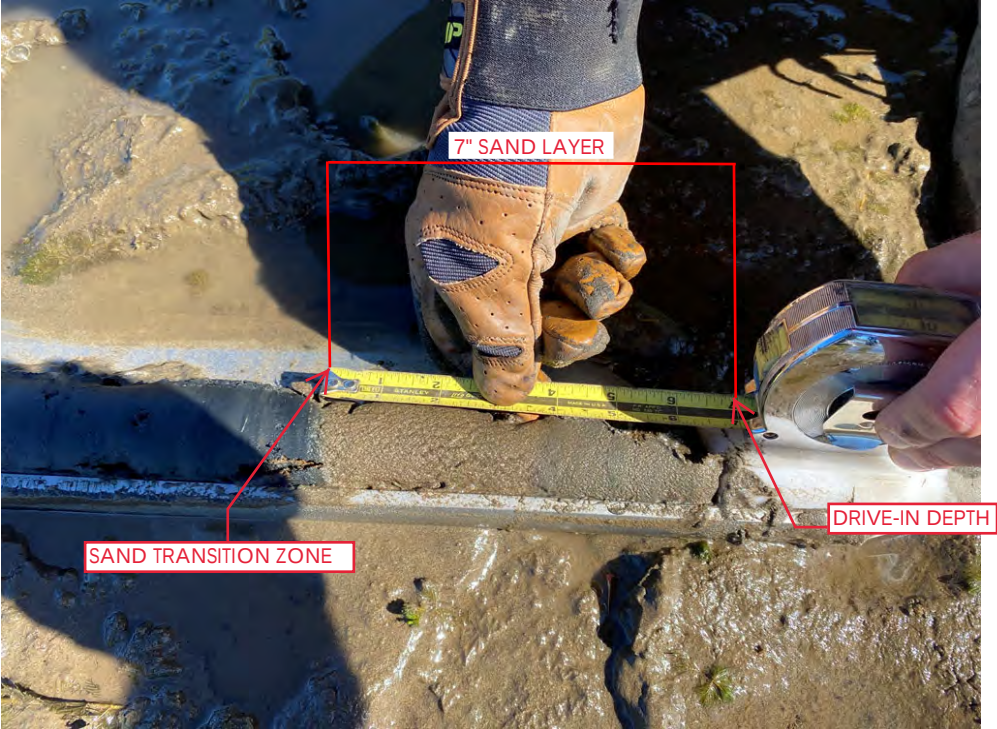
Photo 14: A look at the sampled EMNR Sand profile collected at SP 21, with a depth of approximately 7"
