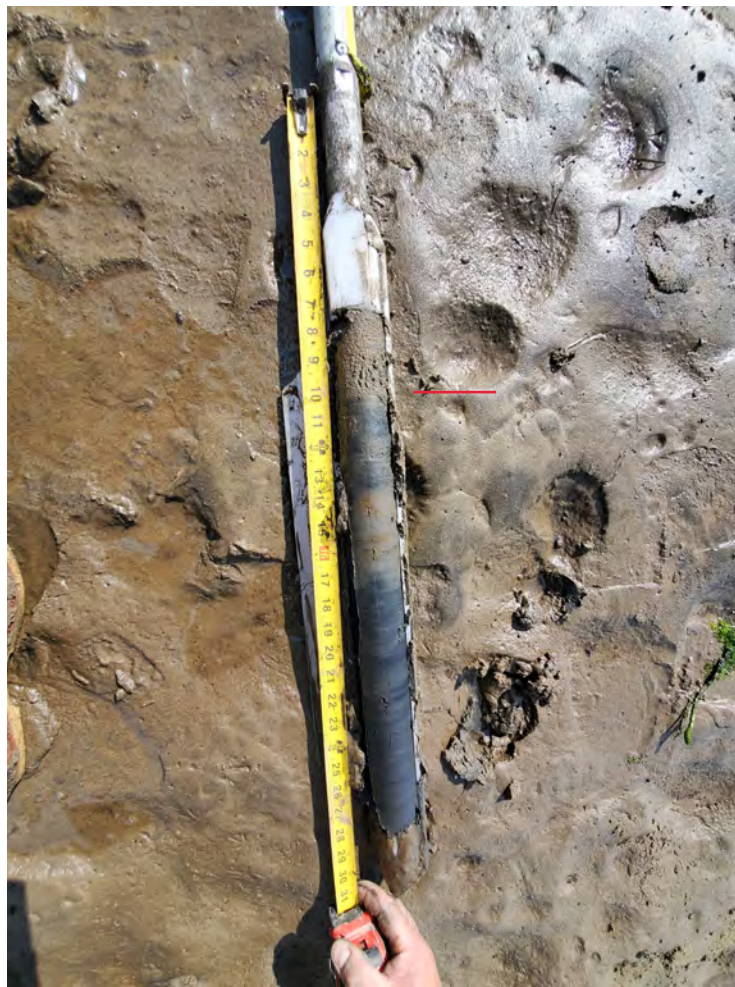
EMNR Sample 9: Photo showing an EMNR layer depth of 10".
