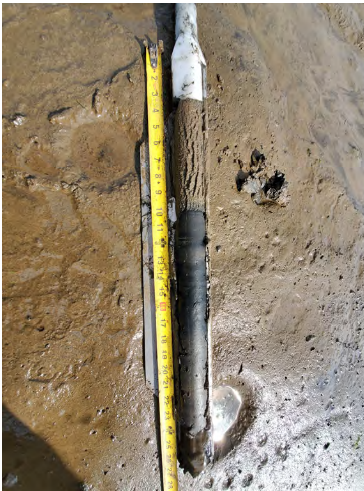
EMNR Sample 7: Photo showing a sand layer thickness of 10".
