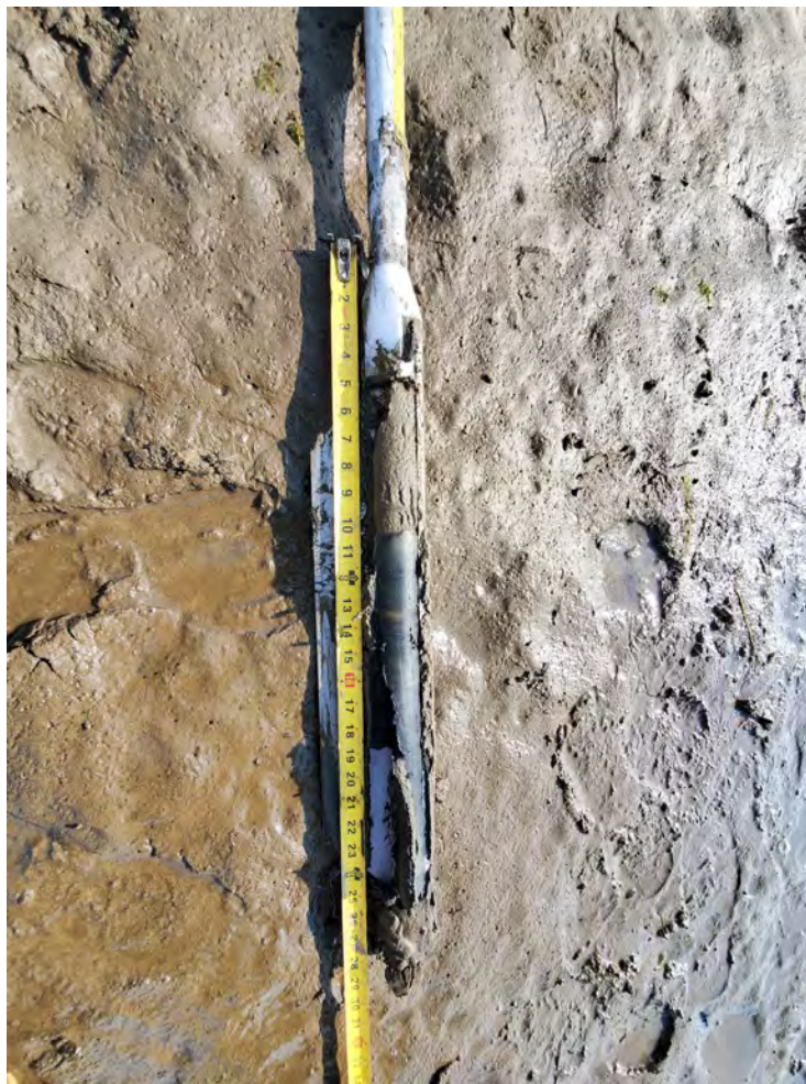
EMNR Sample 3: Photo showing a sand layer thickness of 10".
