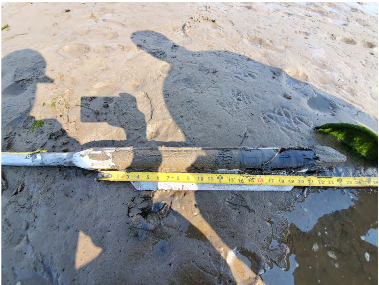
EMNR Sample 5: Photo showing a sand layer thickness of 14".
