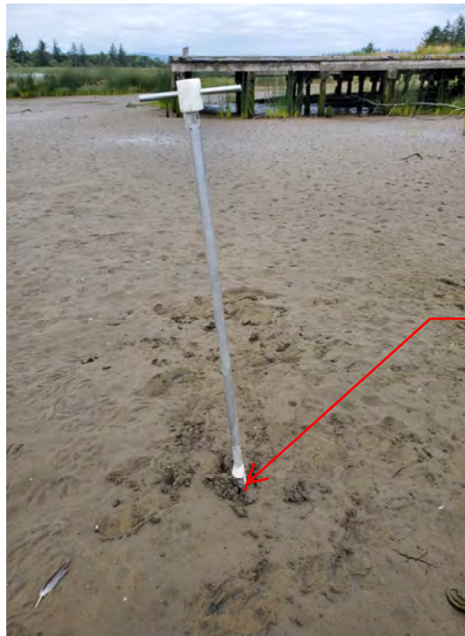
Photo 14: A look at the drive-in location of the russian pete bore at SP-12
