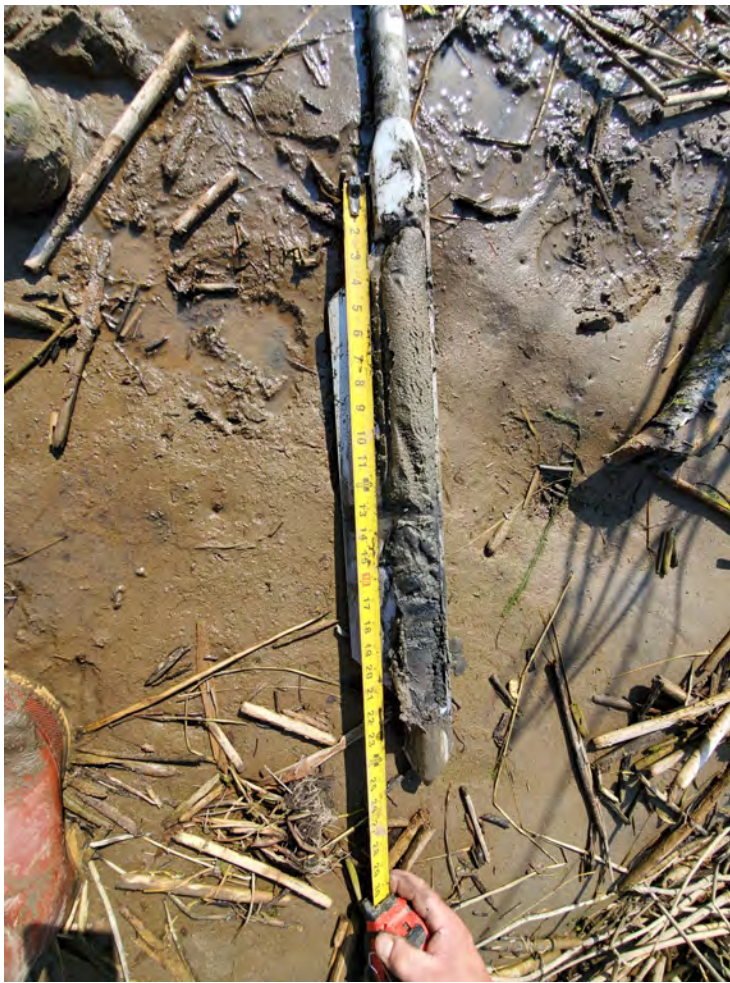
EMNR Sample 10: Photo showing a sand layer depth of 13".
