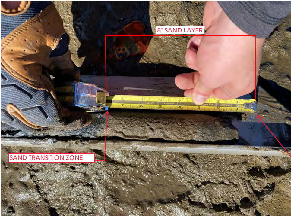
Photo 14: A look at the sampled EMNR Sand profile collected at SP 20, with a depth of approximately 8"
