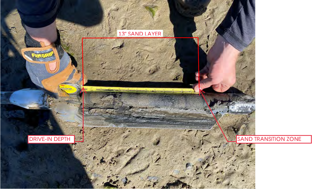
Photo 14: A look at the sampled EMNR Sand profile collected at SP 22, with a depth of approximately 13"
