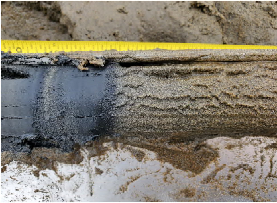
Photo 8: A look at the event horizon (transition zone between sediment and sand) for SP-5
