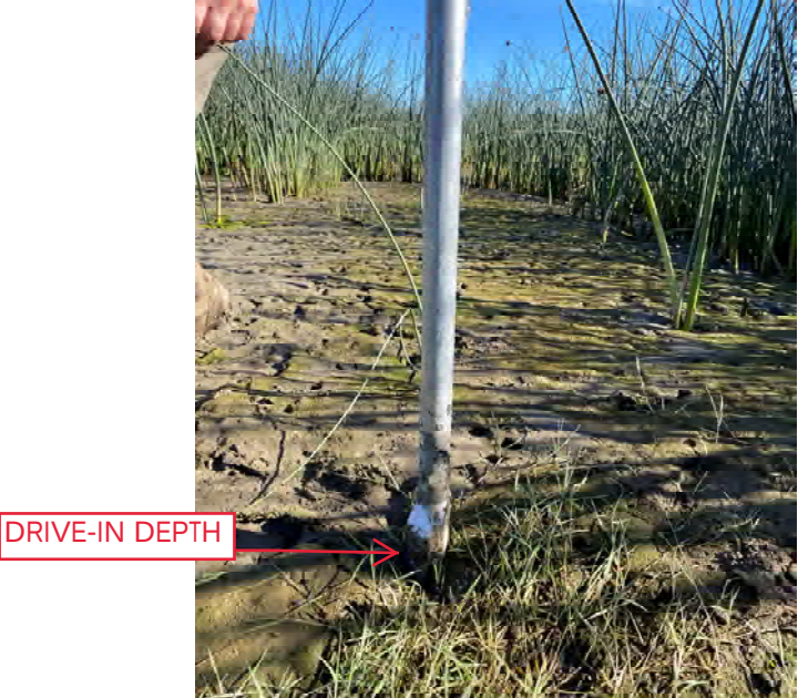
Photo 3: A look at the drive-in location of the russian pete bore at SP 11
