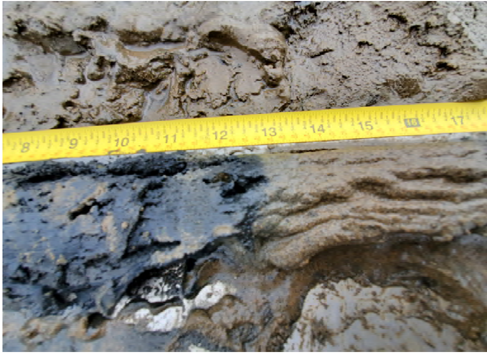
Photo 20: A look at the event horizon (transition zone between sediment and sand) for SP-14
