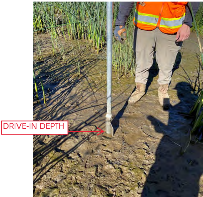
Photo 11: A look at the drive-in location of the russian pete bore at SP 15
