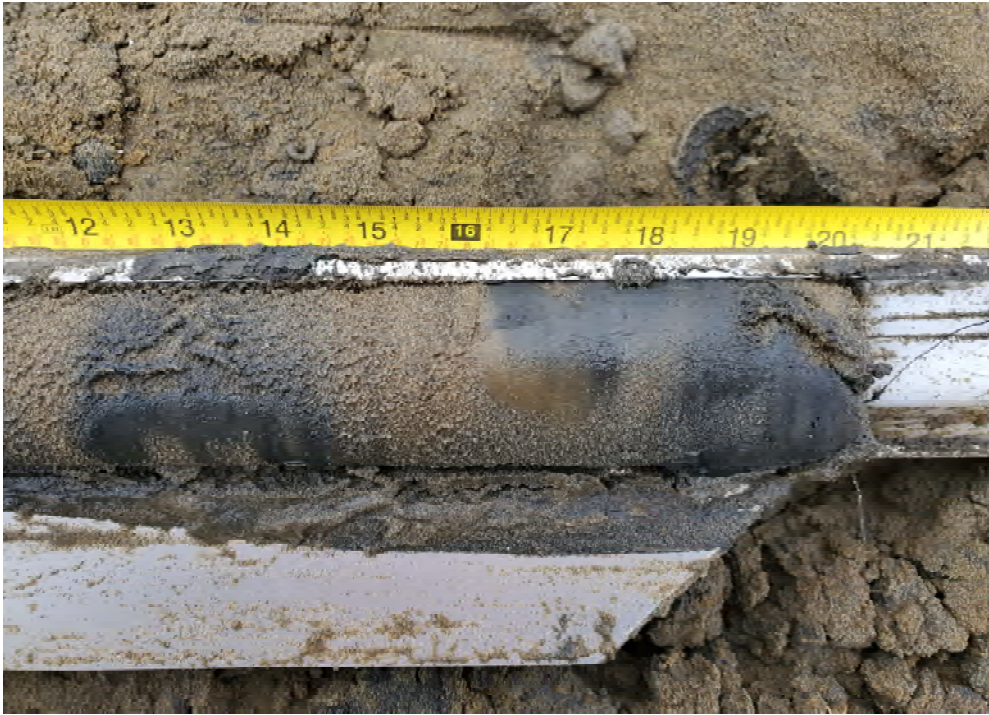
Photo 16: A look at the event horizon (transition zone between sediment and sand) for SP-12
