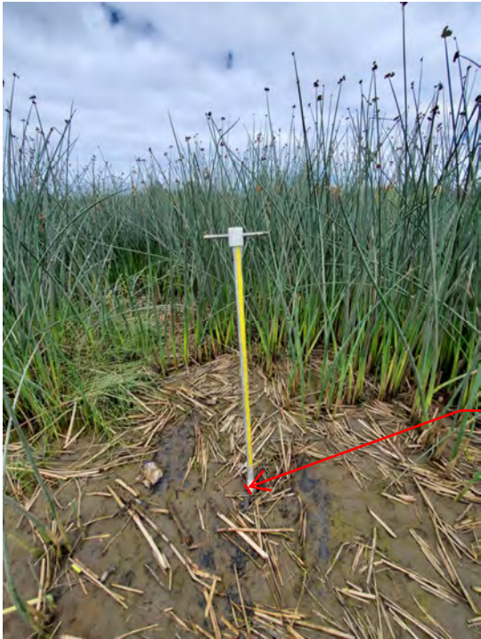
Photo 10: A look at the drive-in location of the russian pete bore at SP-11
