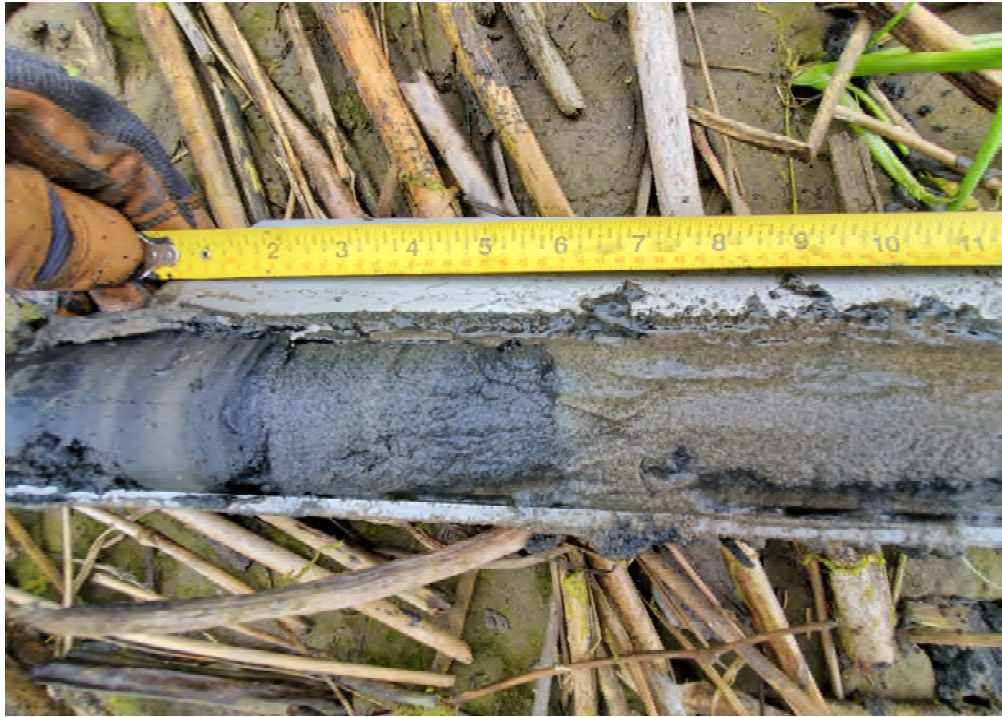
Photo 12: A look at the event horizon (transition zone between sediment and sand) for SP-11
