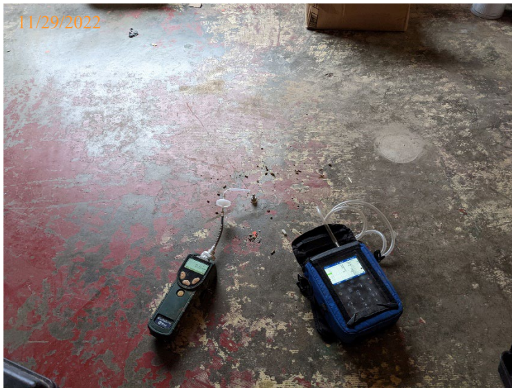
Sub-slab vapor was screened with a PID and GEM 5000 landfill gas meter following sample collection.
