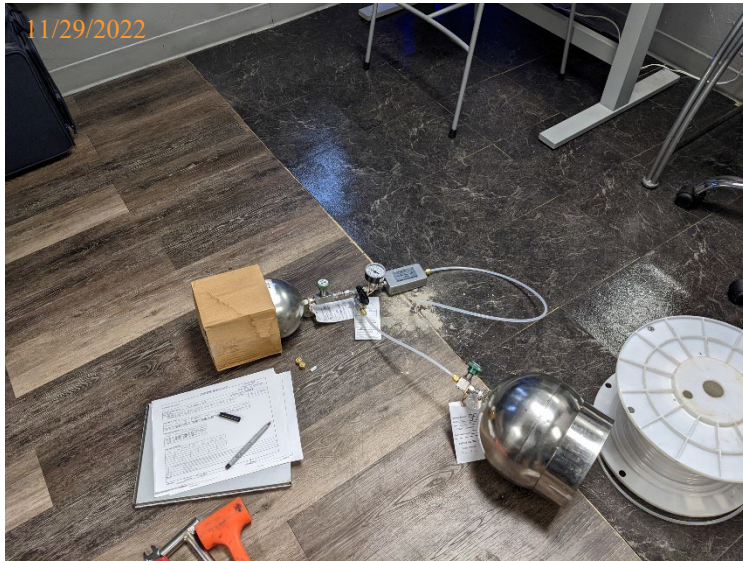
Sampling SUMMA canister (left) and purge canister (right) while purging SUB07.
