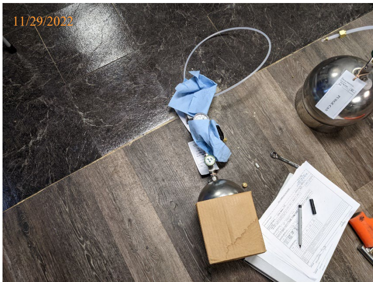
Sampling SUB07. Note IPA saturated blue cloths for leak detection draped over fittings during sample collection.
