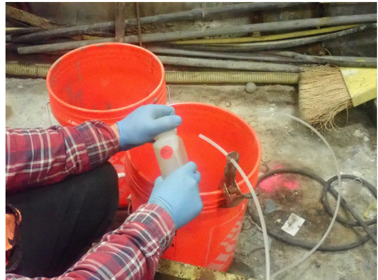
Collecting a pit water sample from EB03.
