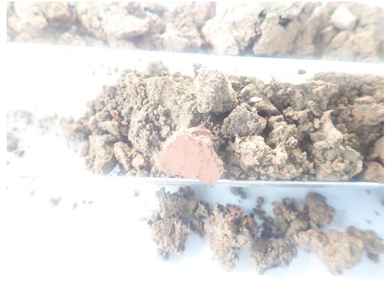
Close-up view of unconsolidated soil materials retrieved from borings.
