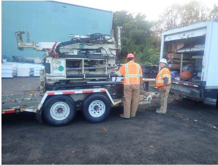
A Geoprobe drill rig was used to advance borings in the southern portion of the site on November 28, 2022.
