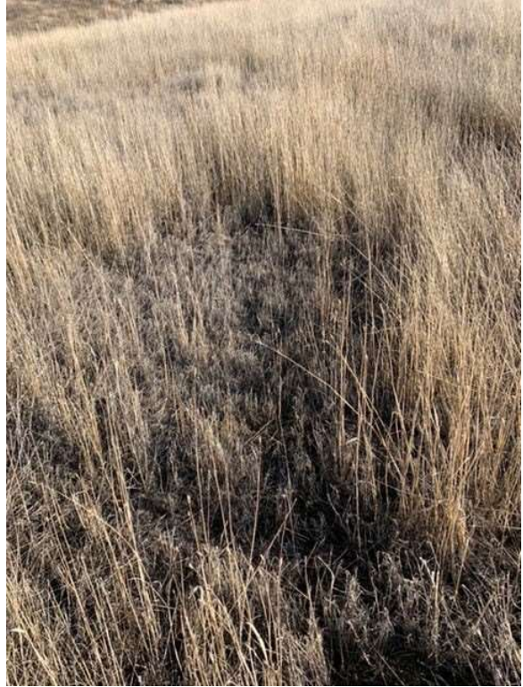
Flattened and dark vegetation on landfill cap
