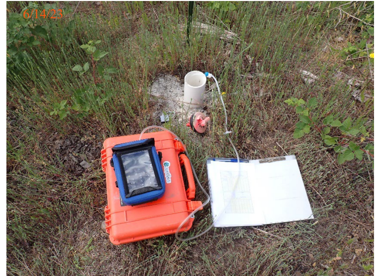
Using a GEM 5000 to monitor a semi-permanent soil gas monitoring point.
