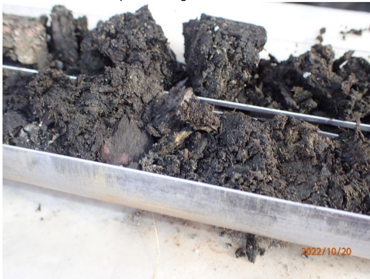
Soil cores were inspected continuously, and observations recorded on boring logs. Particular attention was given to soils containing organic matter.
