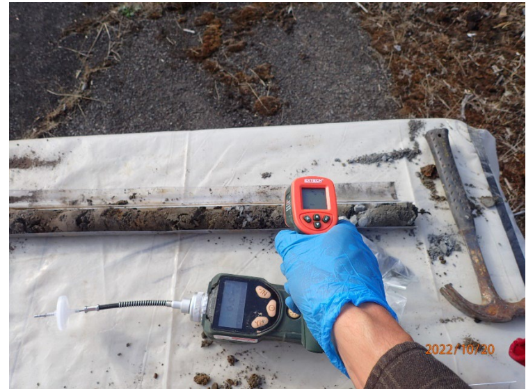
A photoionization detector and laser thermometer were also utilized to screen soil cores for possible indications of methanogenesis.
