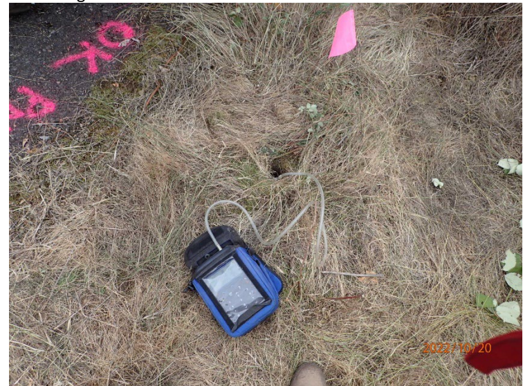
Immediately upon reaching total depth, open boreholes were screened for the presence of methane using a GEM 5000.
