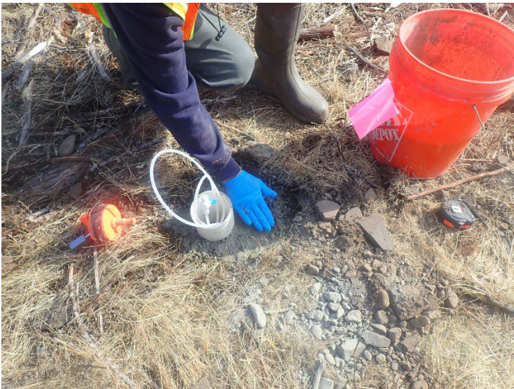
Monitoring points utilized Teflon tubing and a stopcock valve, which remain closed between monitoring events.
