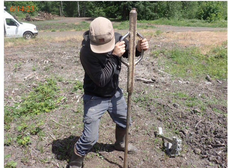
Advancing a temporary soil gas monitoring point using a slide hammer to drive manual soil gas tooling.
