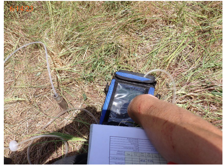
Using the GEM 5000 to monitor soil gas in a temporary soil gas probe (typical).
