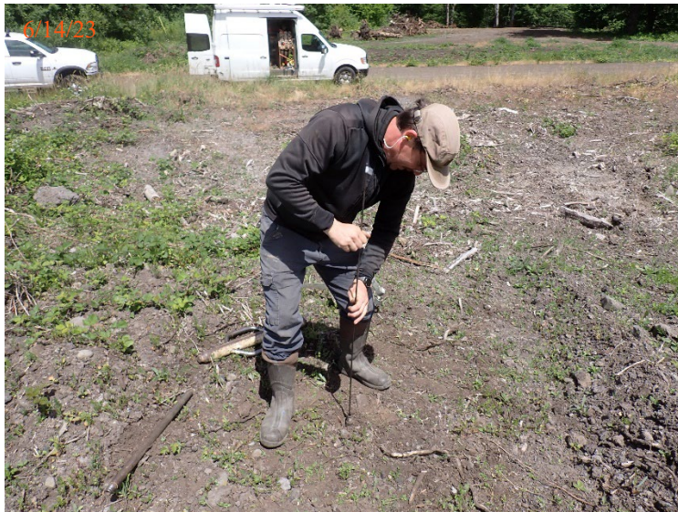
Opening the sacrificial drive tip in preparation for monitoring soil gas.
