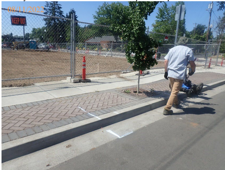
Using ground-penetrating radar to locate the former filled UST cavity midway along the SW side of Arthur Street.
