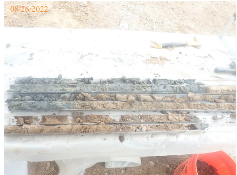
View of soil core from B02, retrieved inside plastic liners and cut open for inspection. 0 feet lower right and 15 feet upper left.
