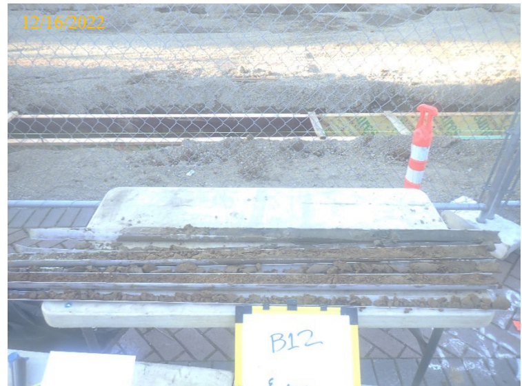
Soil cuttings from 20-foot boring B12 with 0 feet lower right and 20 feet upper left.
