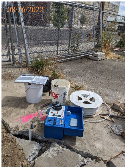
Reconnaissance ground water sampling pump and temporary well casing at B03.
