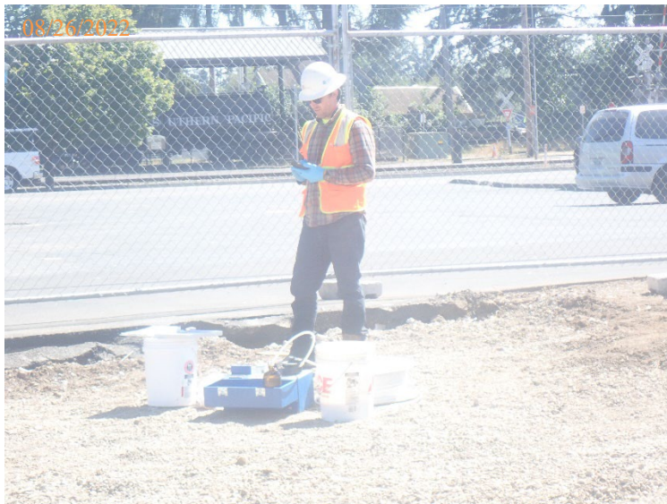
Peristaltic pump used during low-flow purge and sampling of B08.
