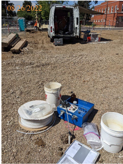
Reconnaissance ground water sampling at B05 – view northwest.
