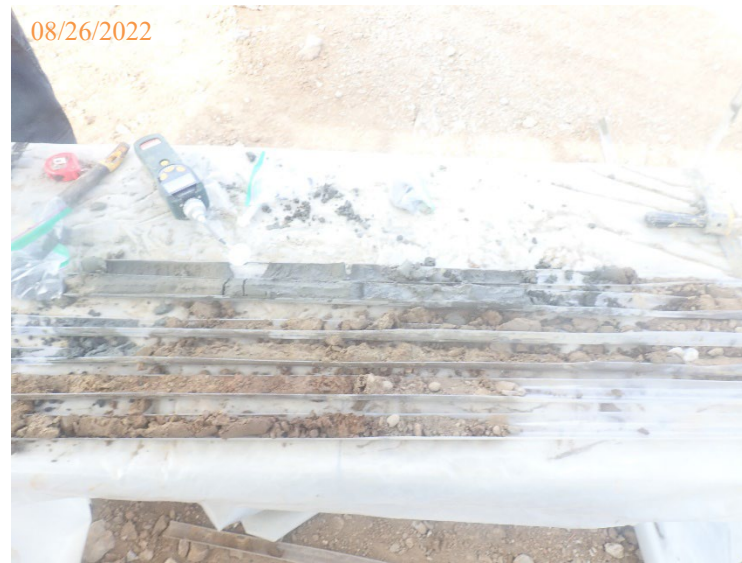
Using a PID to field screen soil core for volatile organic constituents.
