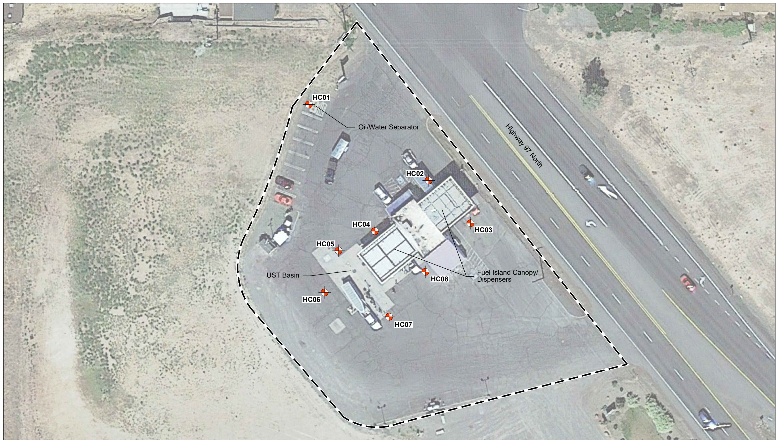
FIGURE 2 BORING LOCATIONS PHASE II ENVIRONMENTAL SITE ASSESSMENT ED STAUB AND SONS 3730 HIGHWAY 97 NORTH KLAMATH FALLS, OREGON
