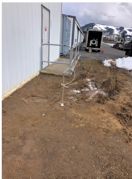
Photo 24. Collecting groundwater in boring 15.
