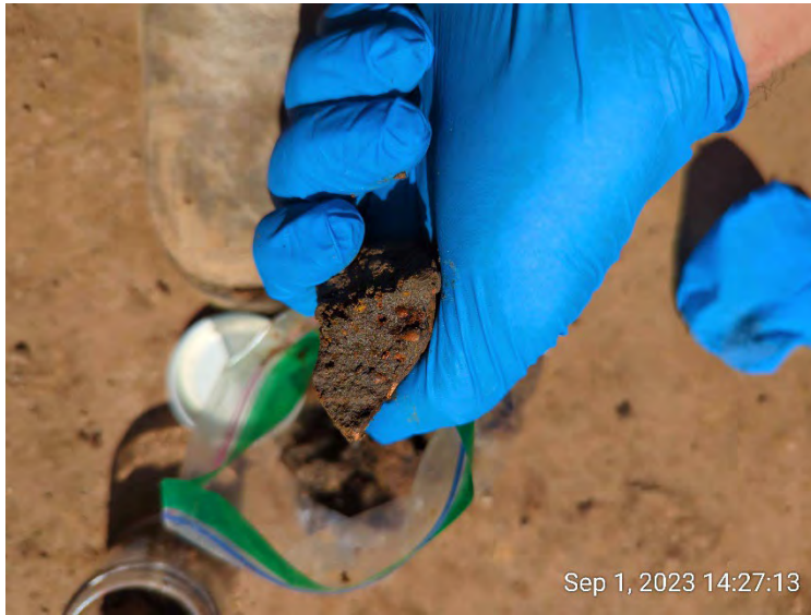
Confirmation grab sample GS01 collected at 14' bgs at the SW corner of EX01. GS02 collected at same position at 12' bgs.
