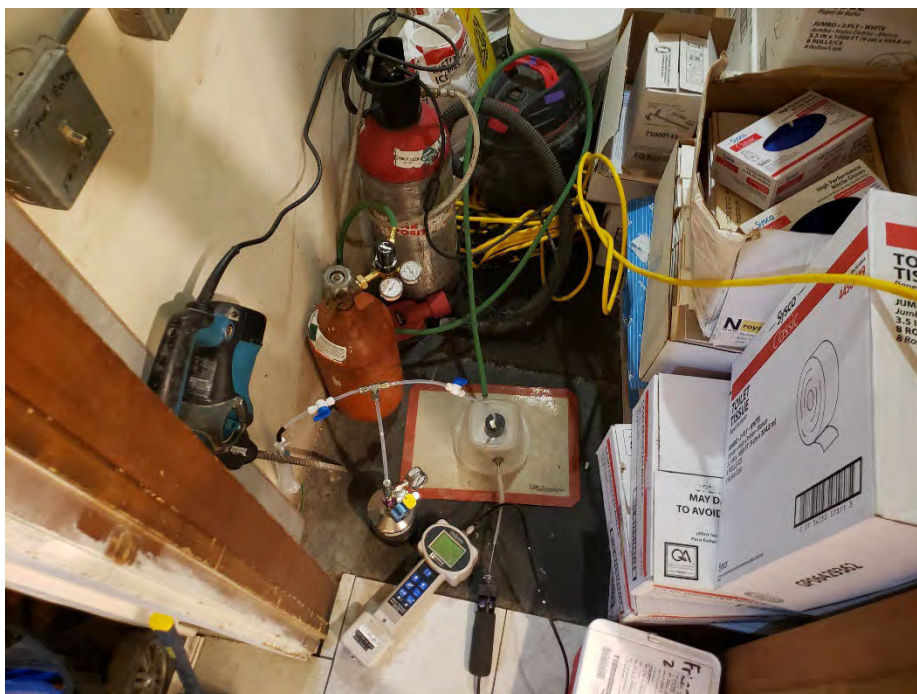
Photo 12. A sub-slab vapor sample being collected from the restaurant portion of the building.
