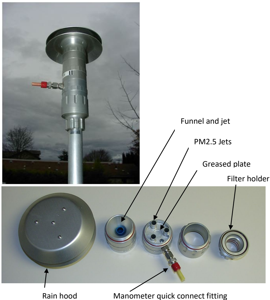
Figure 4. PM 2.5 Inlet with smart manometer connection.
