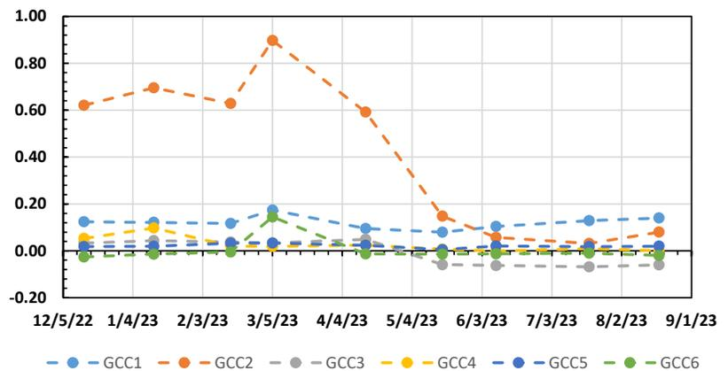
Positive horizontal gradient indicates an inward hydraulic gradient across the GWB.
