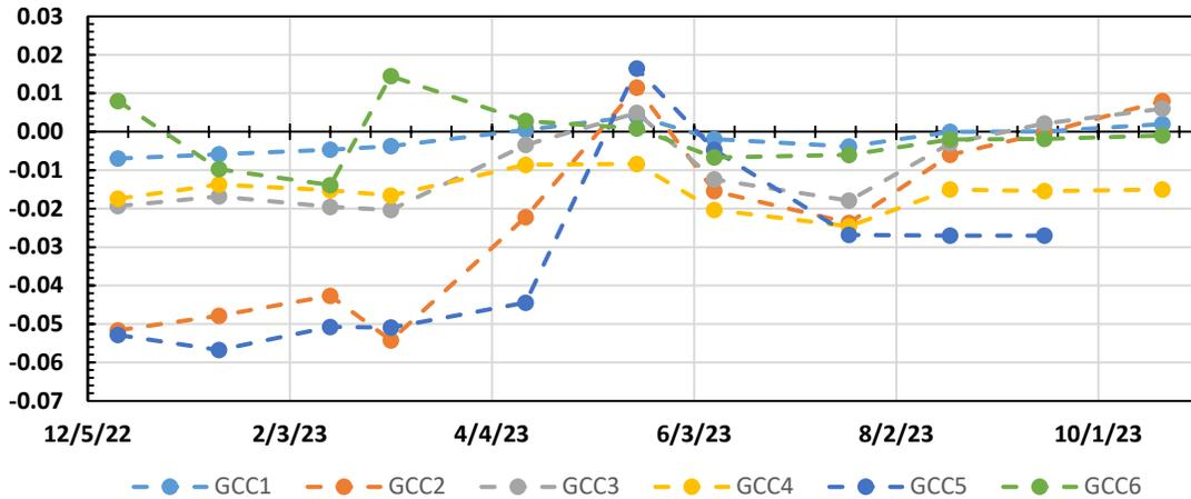
Positive horizontal gradient indicates an inward hydraulic gradient across the GWBW.
