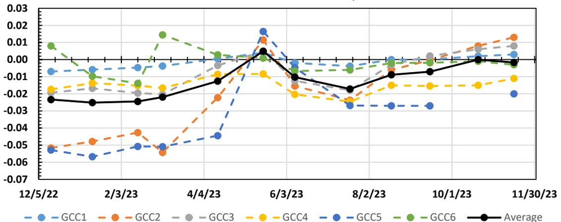
Positive horizontal gradient indicates an inward hydraulic gradient across the GWBW.
