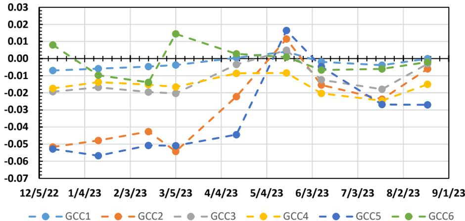
Positive horizontal gradient indicates an inward hydraulic gradient across the GWBW.
