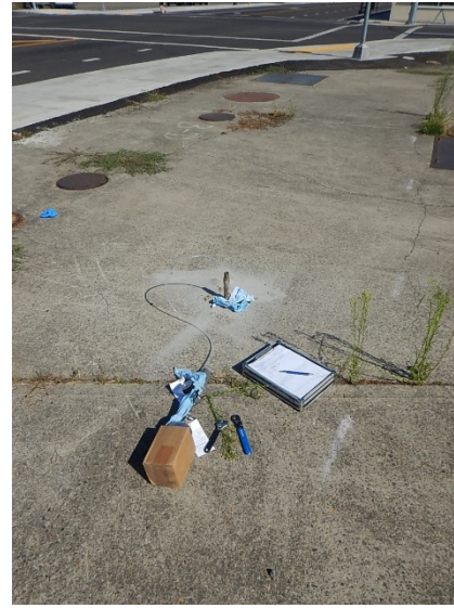
View north of soil gas sample SG01, located just south of the existing USTs (note placement of rags saturated with IPA for leak check).
