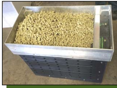
Refilling tray on cartridge with bulk media.
