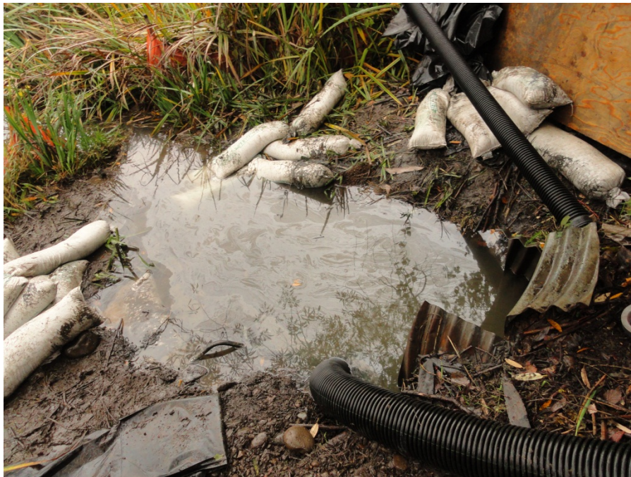
P-2: Sheen was observed at the outfall entering Johnson Lake.
