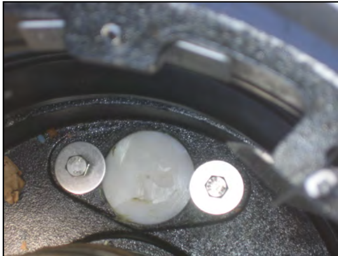
Figure 1-4 1DP-2100 Field Installed Drain Plug
