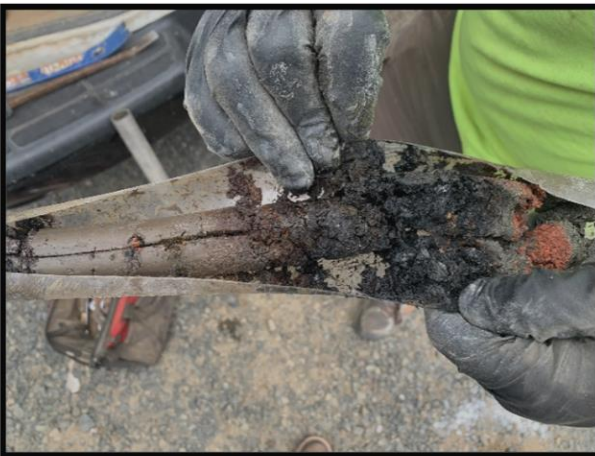
PHOTOGRAPH NO. 5 – Asphalt cuttings in fill material observed in Boring B4.
