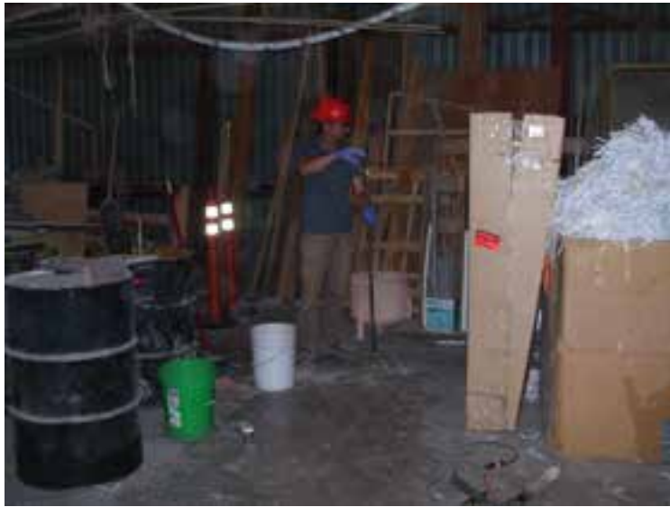
View of sampling inside the building using a stainless-steel hand auger.
