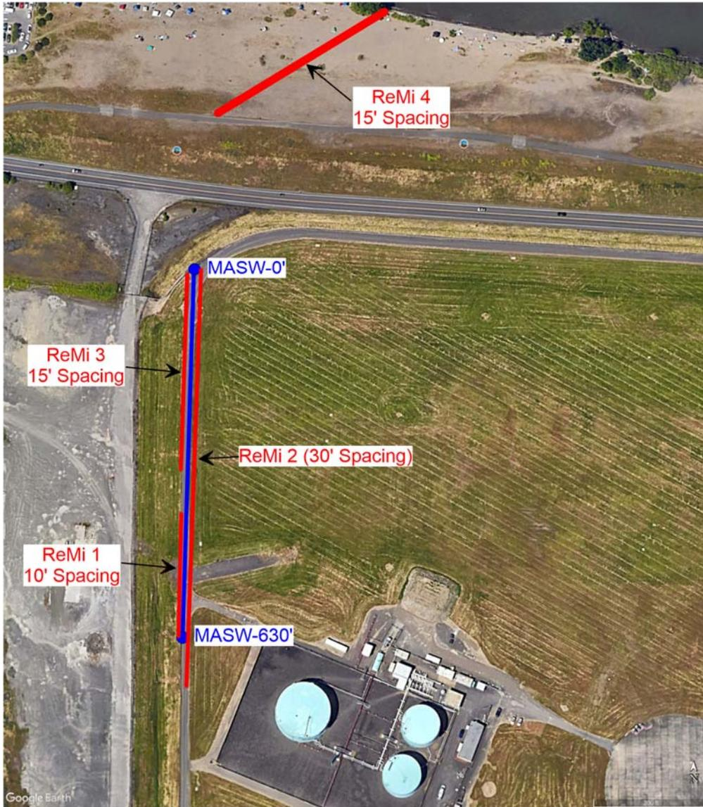
Figure 2-1. Site layout showing locations of geophysical arrays.
