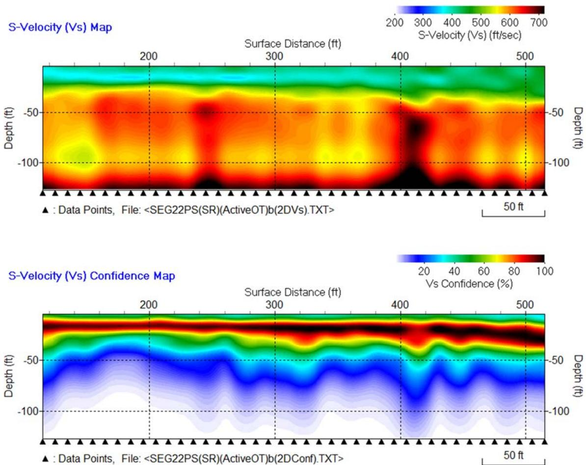
**Figure 4-5. 2-D (top) Vs models and Confidence plot (bottom) from active source MASW Array.**
