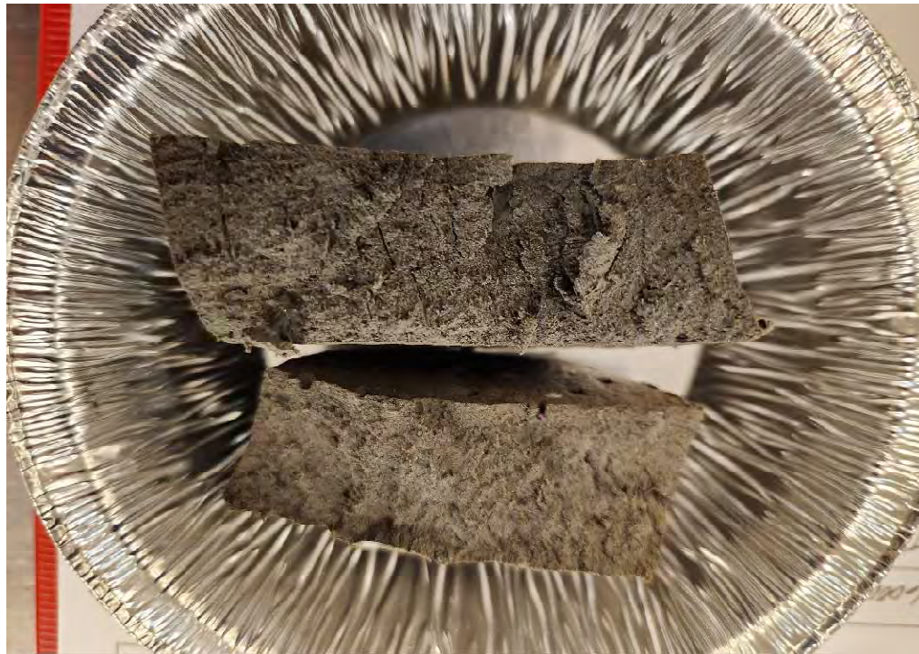
Sample preparation and comments: Thin-walled tube specimen cut from section of tube sample; delaminated and pushed to extrude from tube section.
