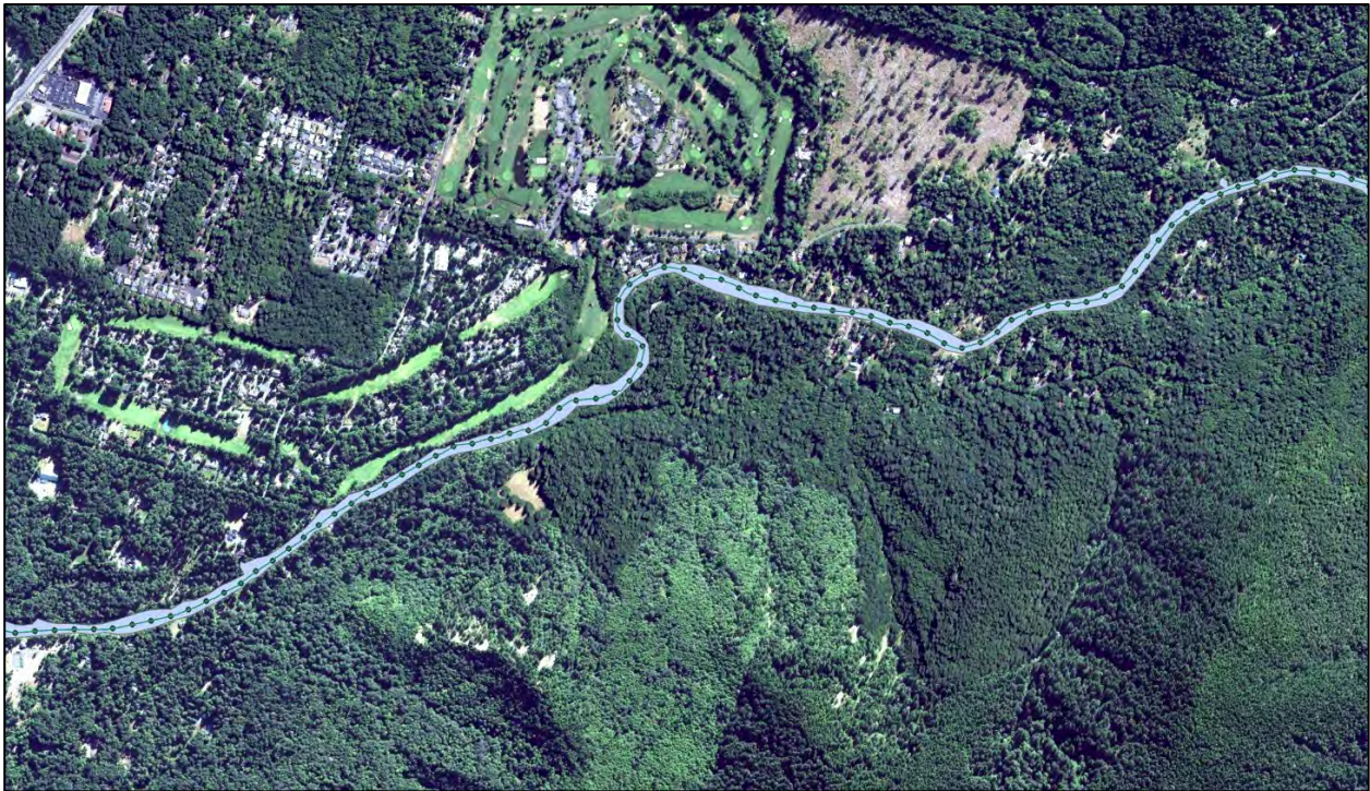
Figure 2-2: Example: Digitized channel (blue line) and stream nodes (green dots) for Heat Source 8.
